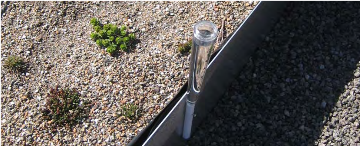
Figure 4-20: Rain gauge at PS118 in Queens.
