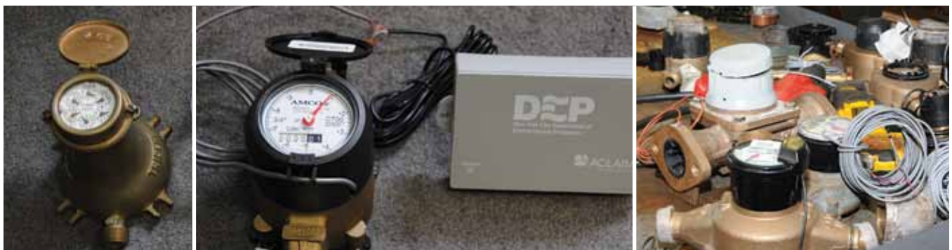
Older water meters were only read four times per year, but wireless meter readers provide real-time data on water use that customers can access online.
