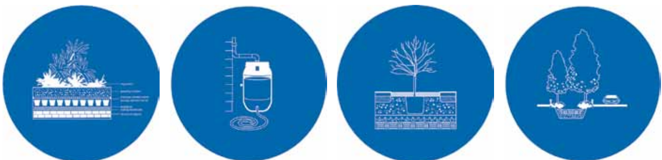
Schematic diagrams of green infrastructure installations show how they capture rain where it falls before it ever enters the sewer system in order to reduce wastewater volumes at our treatment plants. From left: a green roof, a rain barrel, an enhanced tree pit, and a street-side bioswale.
