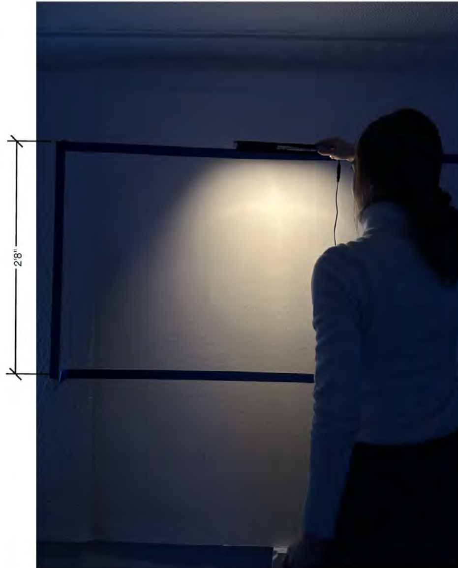
TEST 1: PICTURE LIGHT WITH 12" OFFSET FROM WALL
