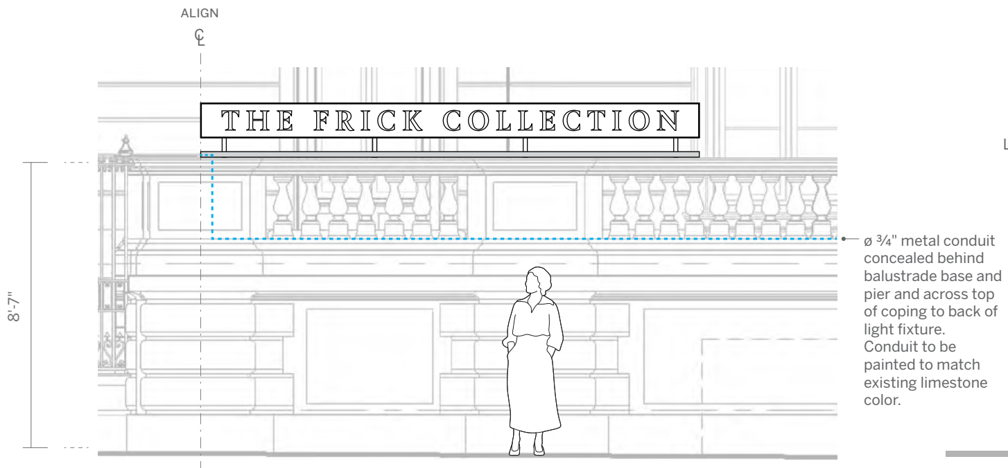
3 West Elevation – Primary Fifth Ave Sign 1/4" = 1'-0"
