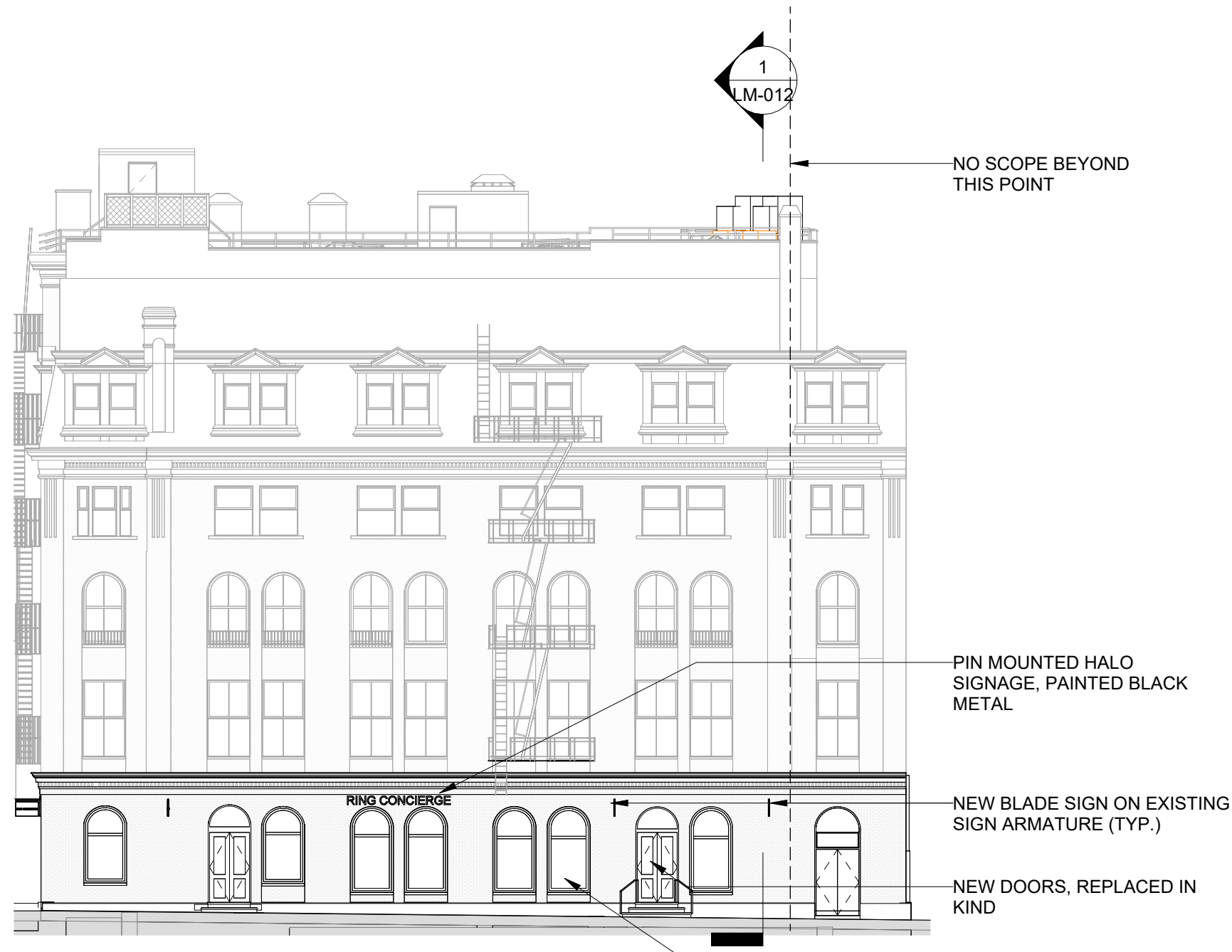
② FACADE ELEVATION - WEST BROADWAY VIEW 1/16" = 1'-0"
