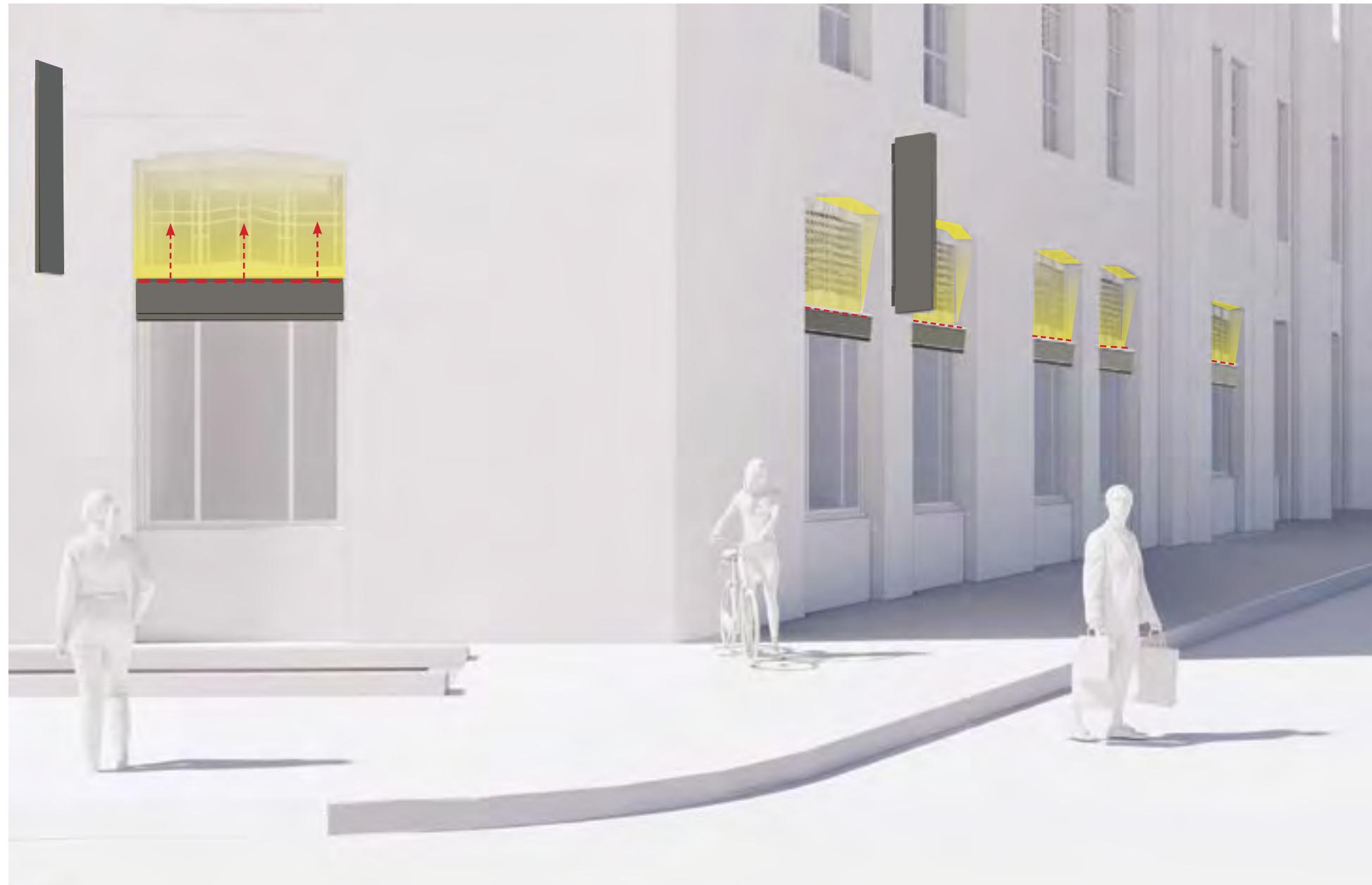
CREATE CONSISTENT LIGHTING DETAIL AT TRANSOMS. MAKE USE OF NEW SIGN BAND TO INSTALL NEW, LOW WATTAGE LED UP-LIGHT TO HIGHLIGHT THE MULLIONS, DECORATIVE GRILLES AND MASONRY ARCHES
