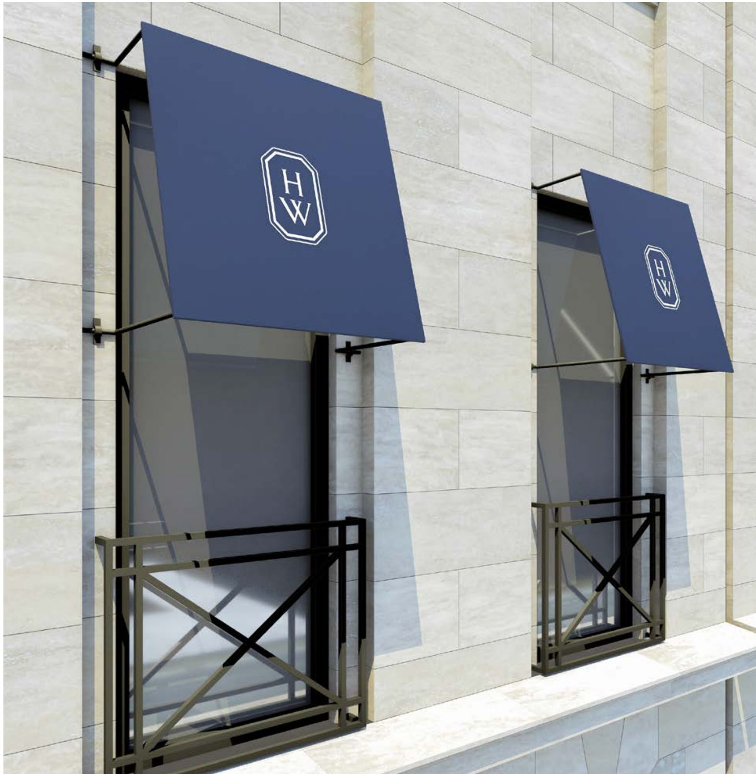
RENDERED VIEW OF WINDOW AWNING AND RAIL
