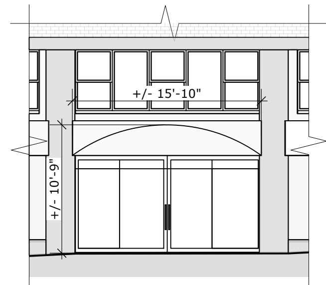
2 MAIN ENTRANCE CANOPY - EXISTING Scale: 1/8" = 1'-0"
