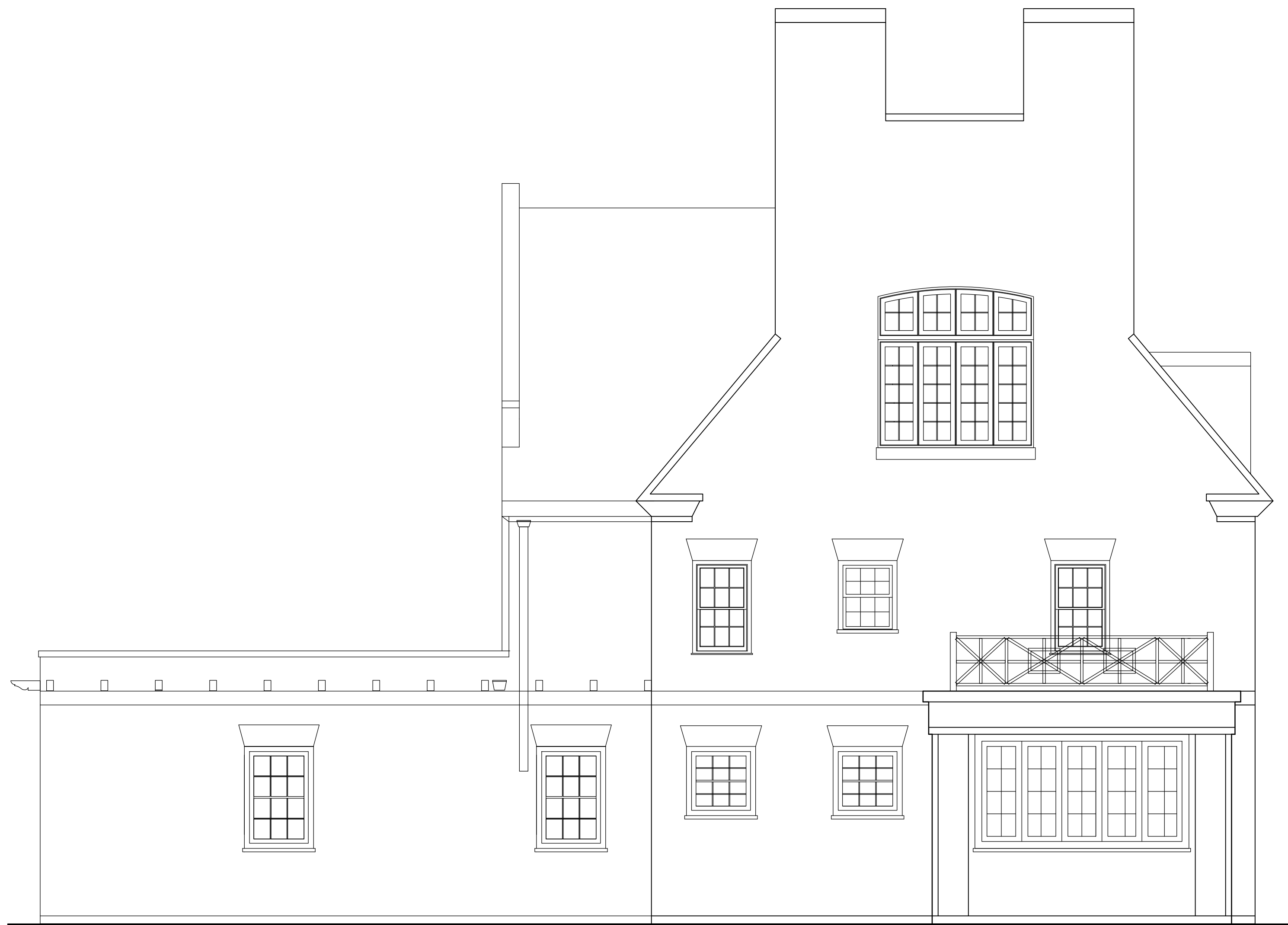
NORTH ELEVATION EXISTING SCALE: 1/4" = 1'-0"
