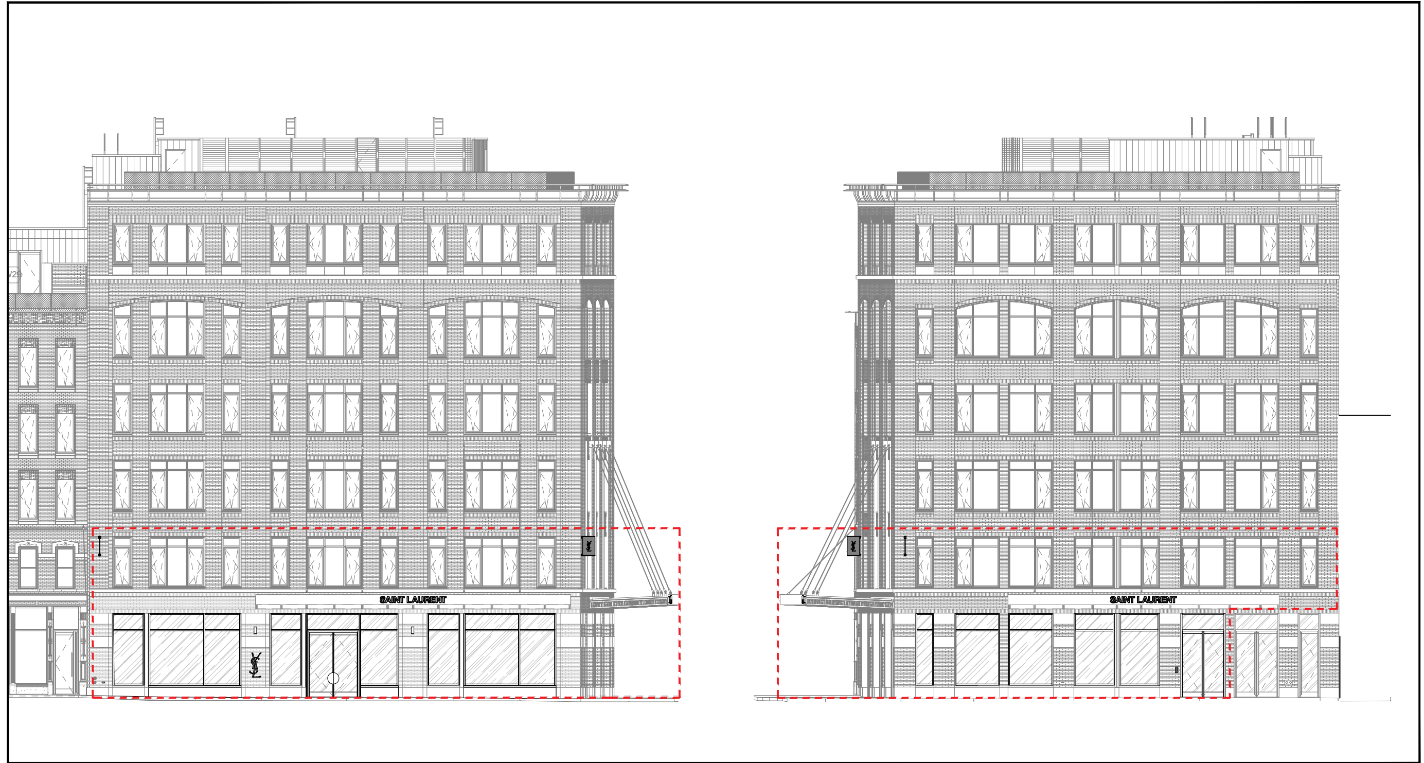
PROPOSED FACADE ELEVATION - GANSEVOORT STREET
