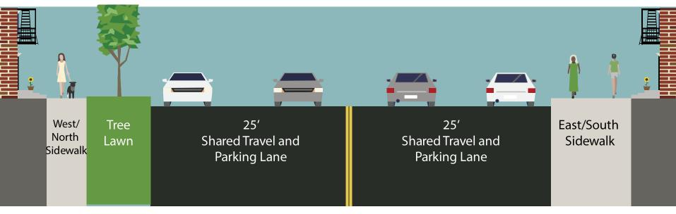
Wide two-way roadway with one moving lane and parking lane in each direction
