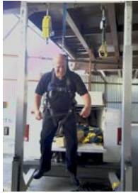
Executive Director of Bridge Preventive Maintenance and Repair Thomas Whitehouse Hoisted in the Air While Wearing a Full Body Harness - Demonstrating How to Deploy and Use the Foot Stand to Prevent Orthostatic Intolerance (Commonly Referred to as Suspension Trauma), Which Can be Fatal if Not Prevented. (Credit: Gean Pilipiak)
