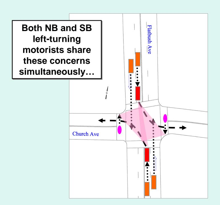
Separation of left and thru movements on Flatbush Avenue to prevent left turning vehicles from blocking traffic on Flatbush while waiting for a gap
