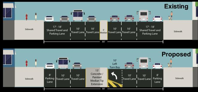
Construct 10 concrete median tip extensions
