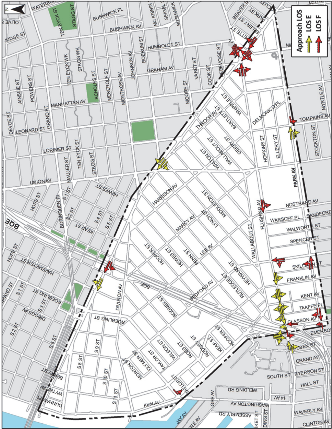
Figure 4-7: Existing Intersection Lane Group with LOS E or F –AM Peak
