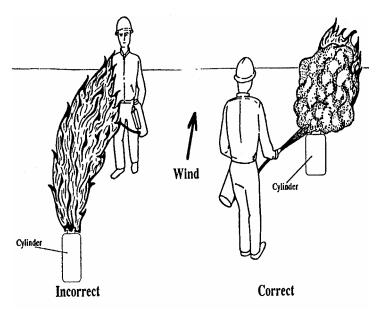
The dry chemical stream must be directed toward the point where the flame begins. Do not direct the chemical stream at the center of the flame. This will not extinguish the fire. The correct way to direct the dry chemical stream is shown below.
