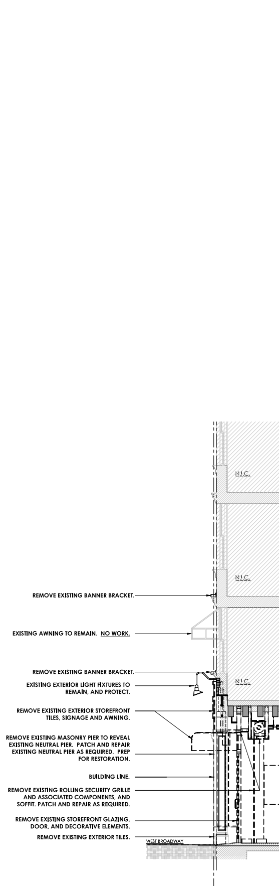
3 SECTION @ DOOR - DEMOLITION 1/4"=1'-0"
