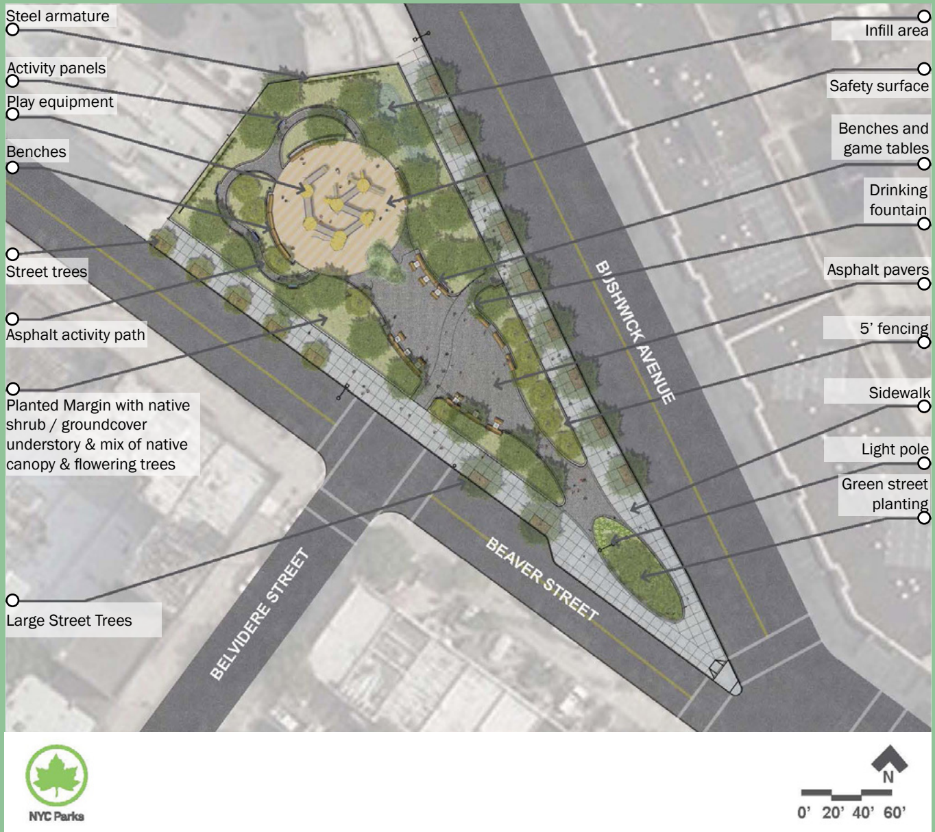
Schematic design for Beaver Noll Park, a new park on Beaver Street and Bushwick Avenue.
