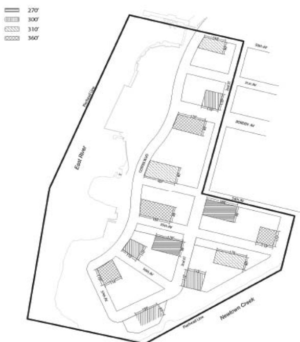
Special Southern Hunters Point District Map 5. Mandatory Sidewalk Widening and Publicly Accessible Open Area
