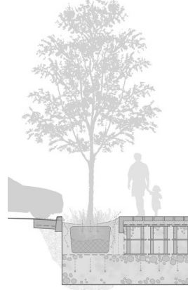
Figure 4.12. Illustration of a hybrid system that incorporates bioretention and porous pavement features (image courtesy of SCAPE).
