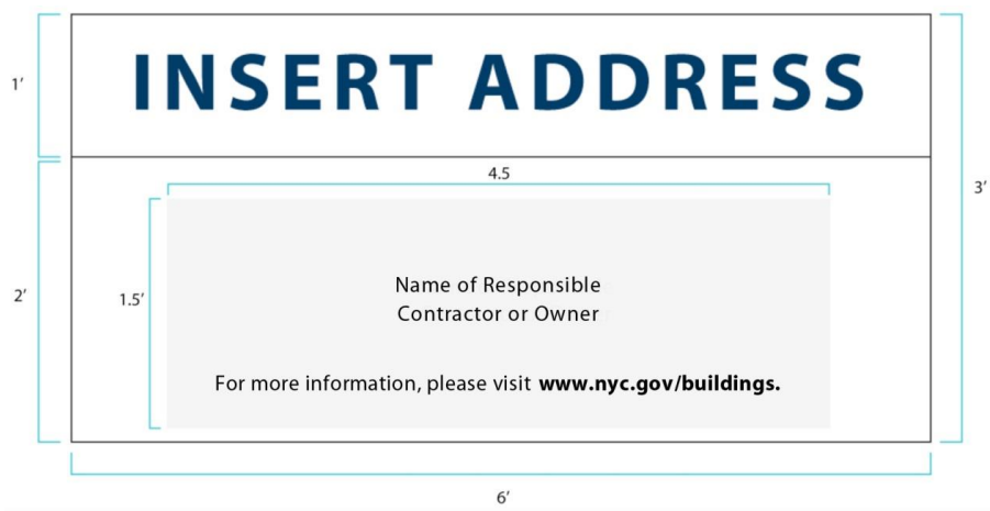
FIGURE 3301.9.2.1(1) SIDEWALK SHED PARAPET PANEL LAYOUT
