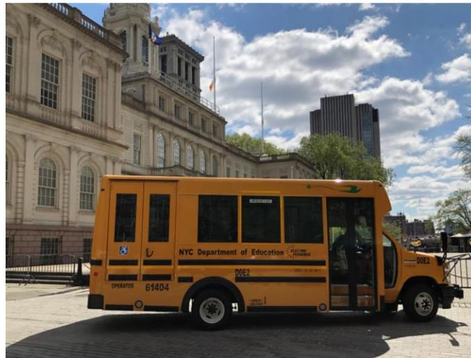
Working with DCAS, the Department of Education (DOE) now has its first two all-electric school busses, both Class A busses, serving up to 20 passengers. Both busses are ADA accessible and will have ranges of 80 to 100 miles per charge. DCAS procured the busses using NY State contracts and is also supplying the electric charging.
