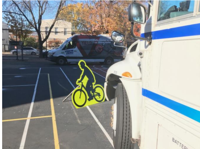
Bicyclist cut out demonstrates line of sight restrictions for truck operators.
