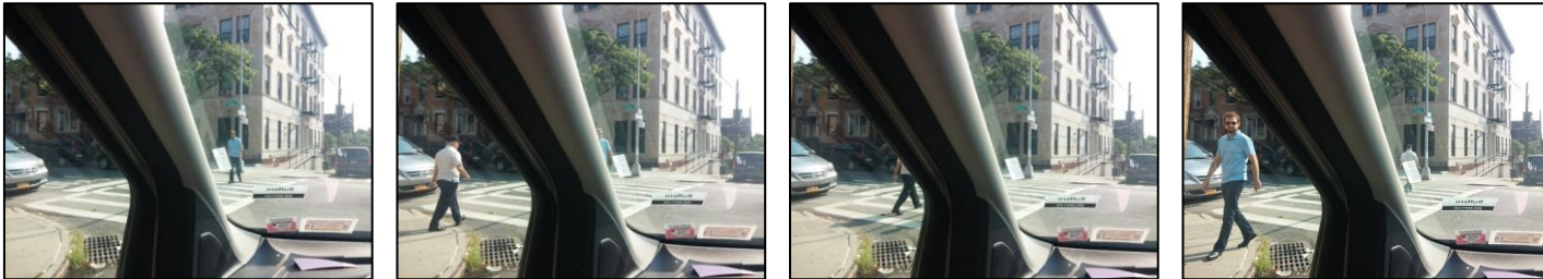
Pedestrians in the crosswalk can disappear behind the vehicle's A-pillar
