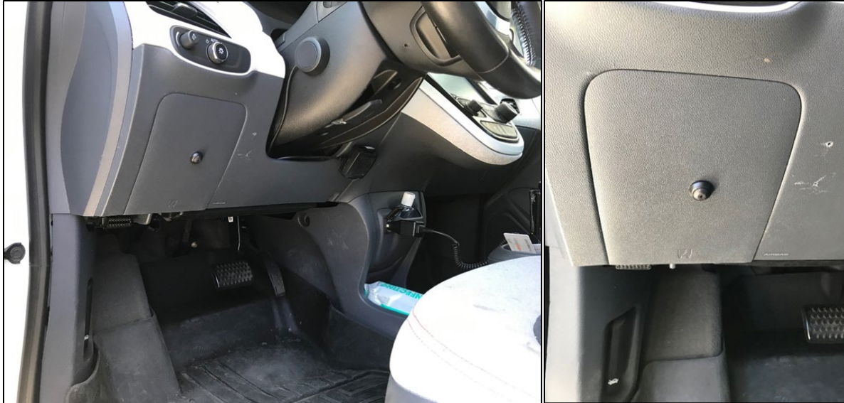
Figure 4. Dashboard/steering wheel area after the ISA install was completed. The driver override button is located on the electrical access panel. (Source: NYC DCAS)
