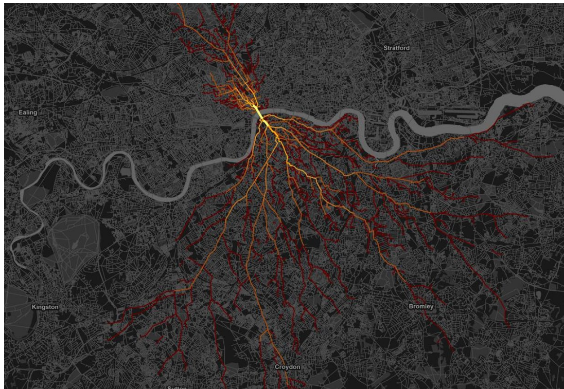
Example model: Transport for London Cynemon cycling model, AM trips using Waterloo Bridge
