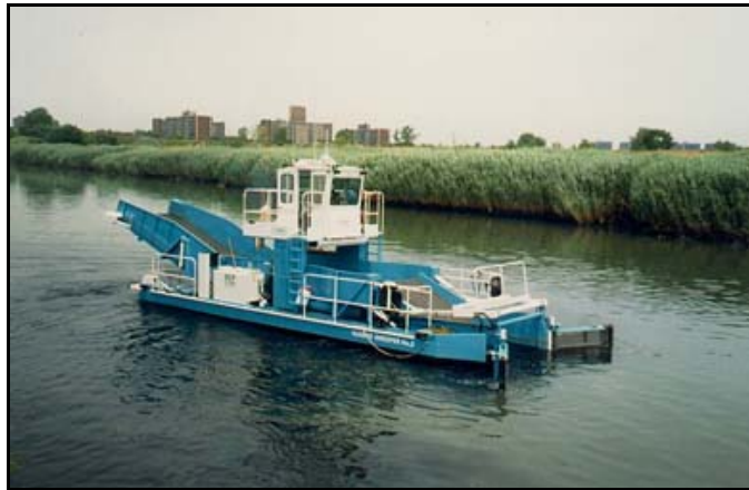
Figure 5-2. UMI TrashCat™ skimming back bay wetland areas of New York City's Jamaica Bay
