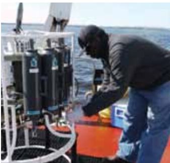
Marine Sciences crew monitors water quality aboard harbor survey research vessel Osprey
