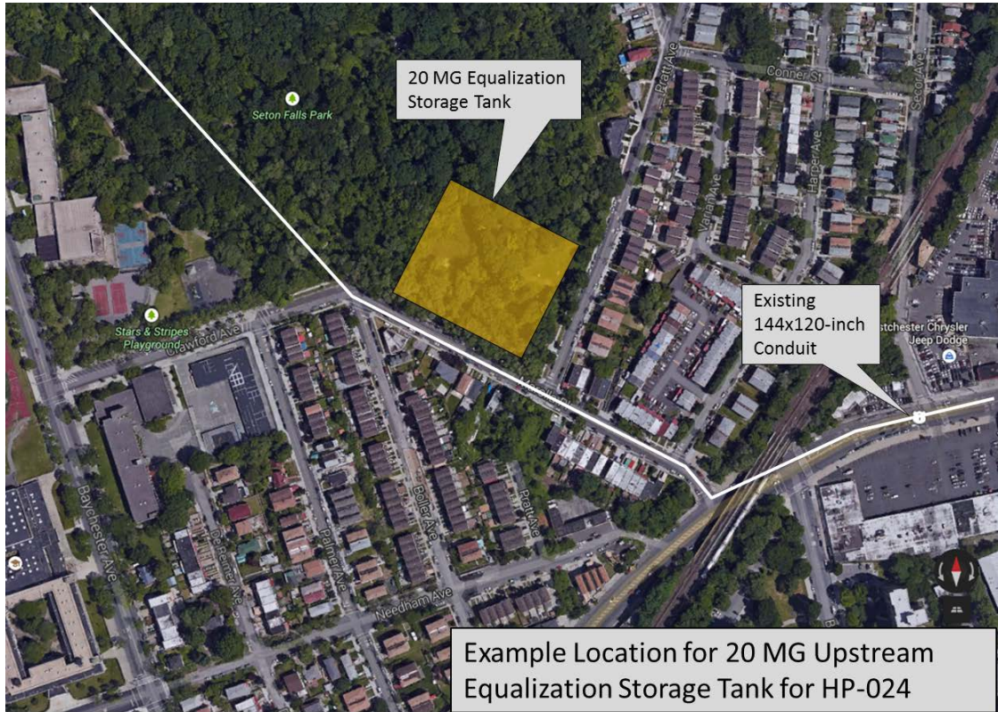
New Figure E-8-2. Siting Option for Upstream Equalization Storage Tank for HP-024- Parkland
