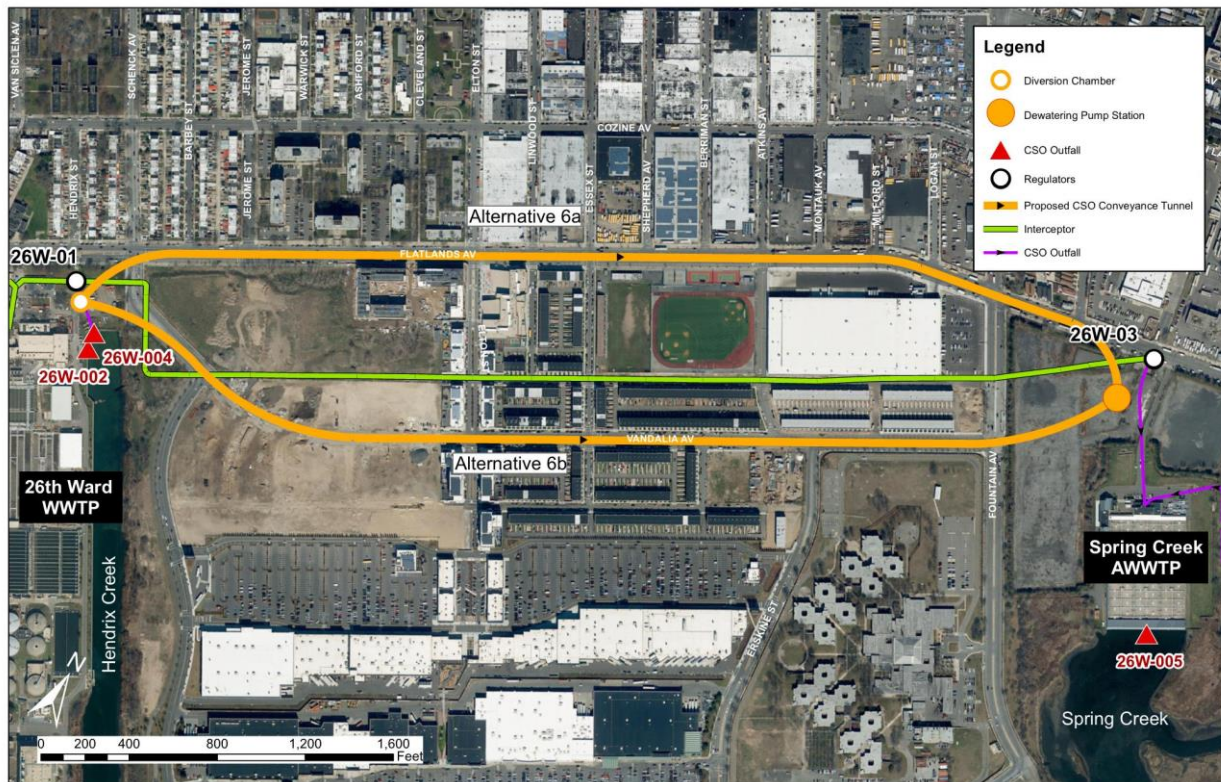
Figure 8-21. Layout of CSO Storage Tunnel and 50 MGD Dewatering Pumping Station at the Spring Creek AWWTP
