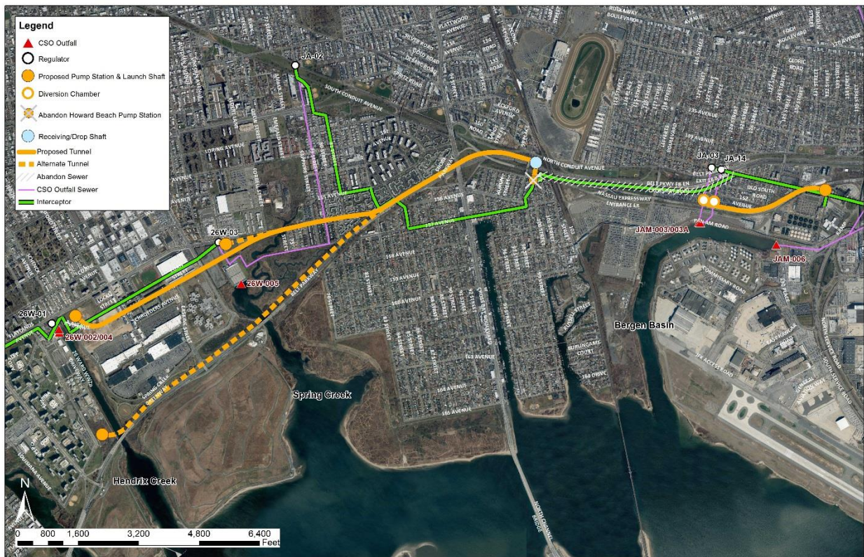
Figure 8-8. Layout for Proposed Parallel Interceptor to Jamaica WWTP and Gravity Sewer to 26 th Ward WWTP
