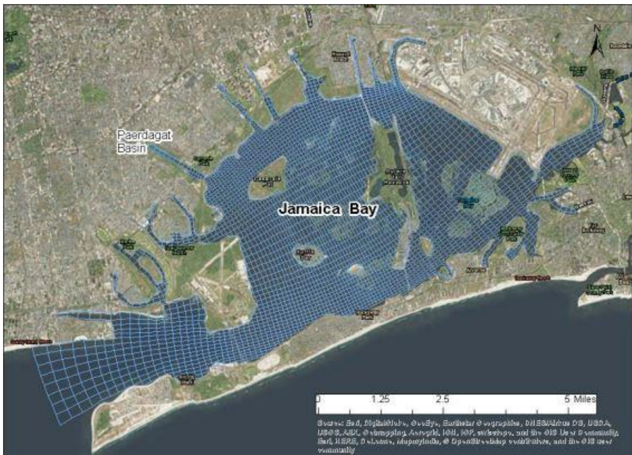
Figure 2-64. Computational Grid for Jamaica Bay Water Quality Modeling
