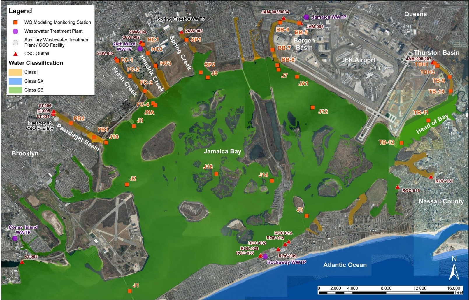
Figure 1. Overview of Water Quality Stations and Permitted Outfalls in Jamaica Bay and its Tributaries
