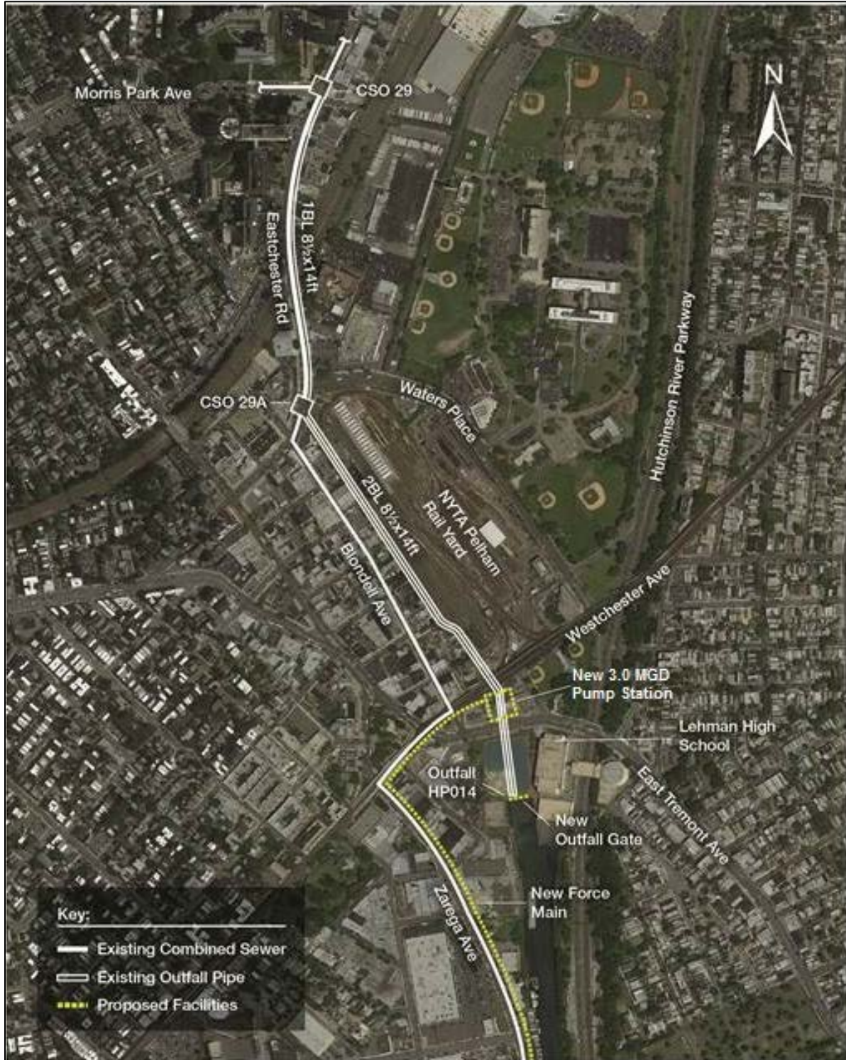
Figure 8-3. Layout of In-line Storage at Outfall HP-014
