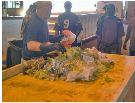
Once the 200 lb sample was brought to the transfer station, it was weighed again and separated into food waste and non-food waste.
