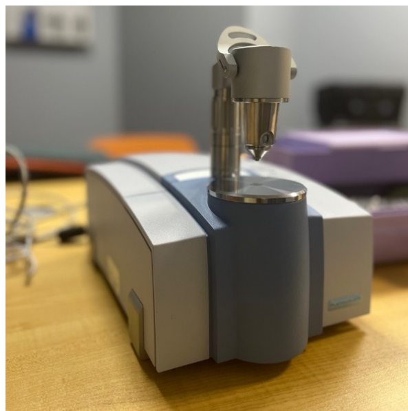
Bruker Alpha II FTIR (photo courtesy of the NYC Health Department's drug-checking team)
