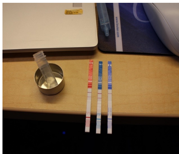
Immunoassay test strips indicating that a drug sample is negative for xylazine (red) and benzodiazepine (blue), and positive for fentanyl (purple) (photo courtesy of the NYC Health Department's drug-checking team)
