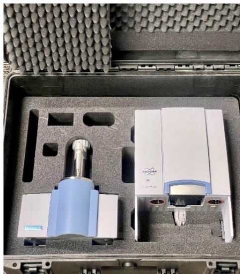
Left: Disassembled Bruker Alpha II FTIR in protective carrying case (photo courtesy of the NYC Health Department's drug-checking team)
