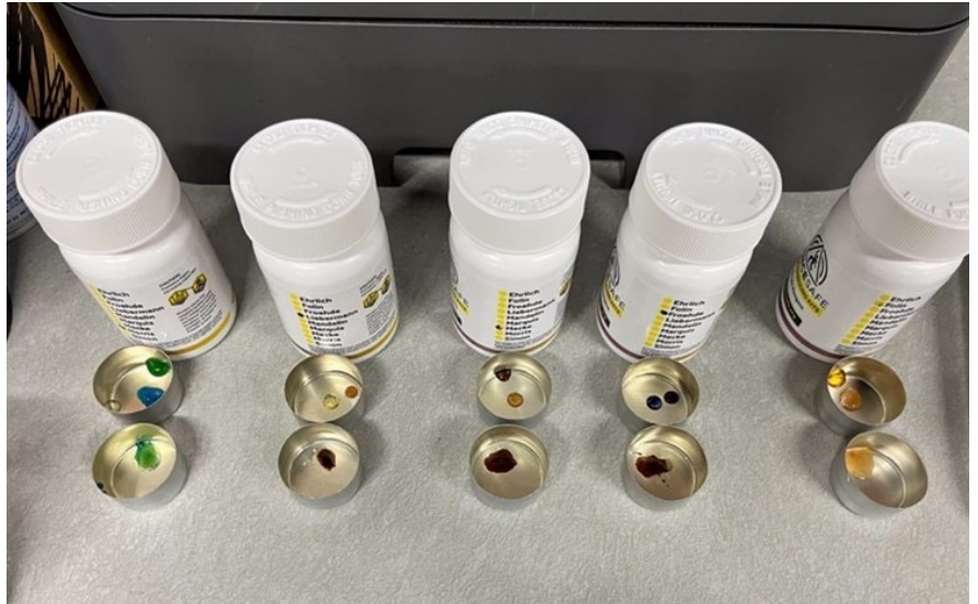
Testing substances in cookers with colorimetric reagents (photo courtesy of Taylor Wood)
