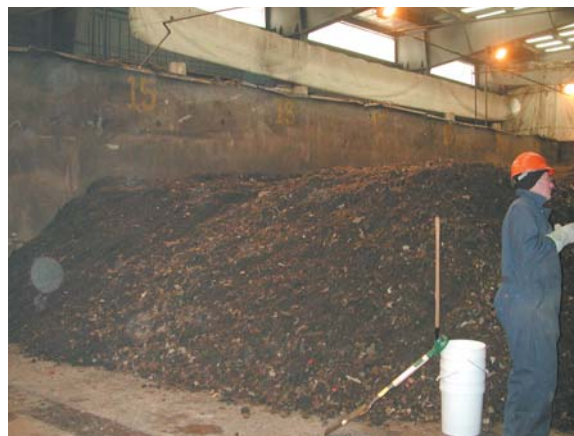
Photo 1-15: Removing samples from the windrows for laboratory analysis
