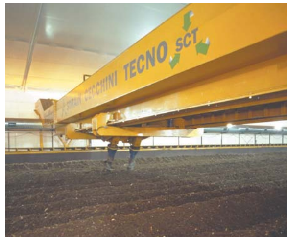
Photo 3-16: Close-up view of an auger mounted on a bridge crane in the Edmonton facility
