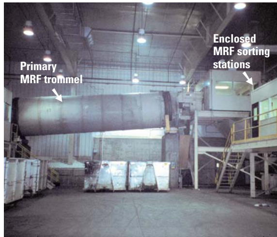
Photo 3-24: Sorting system at the Rapid City MRF
