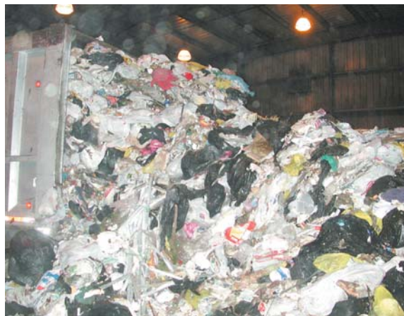
Photo 1-4: Long-haul trucks delivering NYC waste to the Marlborough facility After weighing in, trucks hauling solid waste enter a fully enclosed receiving building and dump their contents onto the tip floor.
