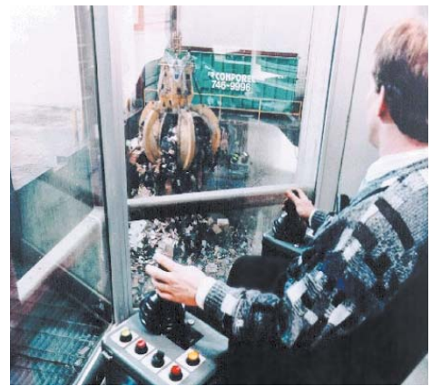
Photo 3-4: Conporec grapple crane operator From the control room, an operator uses a grapple to move waste from the pit to the bioreactor (composting) drum.
