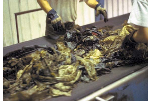
Photo 3-7: Removing recyclables from one-inch overs
