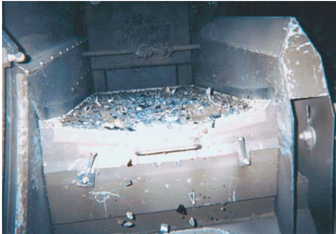
Photo 3-18: De-stoning equipment at the Edmonton facility Upon discharge from the bays, material travels via conveyor to a 25mm (0.985 inch) trommel screen with unders moving to an air classifier. Heavier materials from the air classifier are processed through a de-stoner, which separates compost from contaminants, such as glass and stones (shown above).
