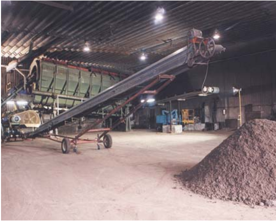
Photo 3-10: Secondary screen at Conporec facility After maturation, the compost moves to a final, five-millimeter screen.
