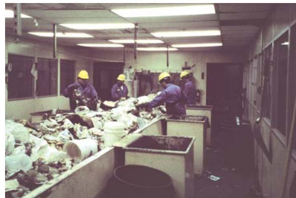
Photo 5-1: Example of an enclosed, climate-controlled sorting station
