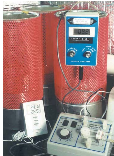
Photo 3-27: Bench-scale reactor The laboratory's bench-scale reactors simulate ideal compost performance by controlling air supply, heat, and moisture. Each bench-scale sample contains approximately four liters of compost.
