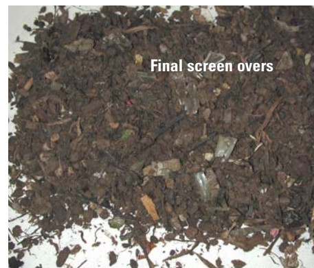
Photo 1-18: Samples of the NYC material passing under (top) and over (bottom) the three-eighths-inch screen
