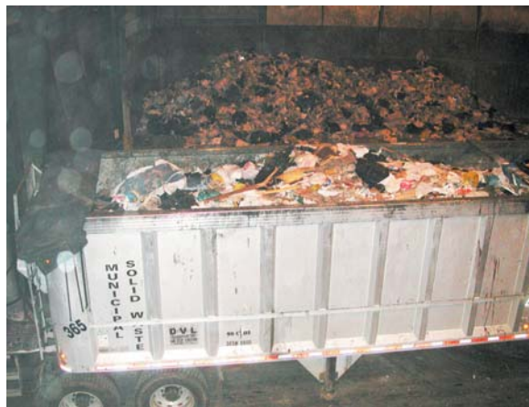
Photo 1-4: Long-haul trucks delivering NYC waste to the Marlborough facility After weighing in, trucks hauling solid waste enter a fully enclosed receiving building and dump their contents onto the tip floor.
