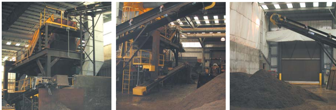
Photo 1-17: Marlborough final-screening equipment While this equipment successfully removes small pieces of glass and plastic particles, Marlborough facility operators no longer use it because too much usable compost was also passing over the screens and being discarded as residue.
