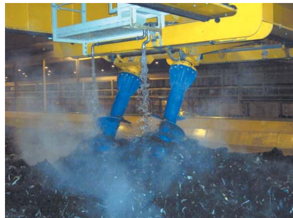
Photo 3-17: A system to add moisture to the composting material on the Edmonton facility air floor
