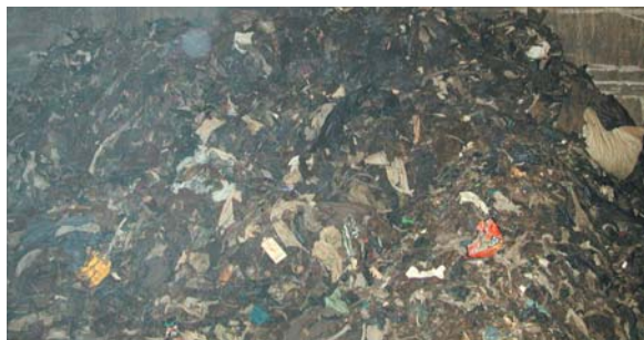
Photo 1-11: Two-inch trommel screen "overs"
