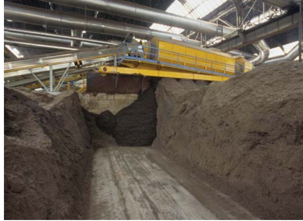
Photo 5-4: Finished compost after final facility screen
