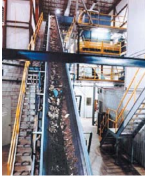
Photo 3-6: Conveyor belt (left) moving material to the Conporec primary trommel screen (right)
