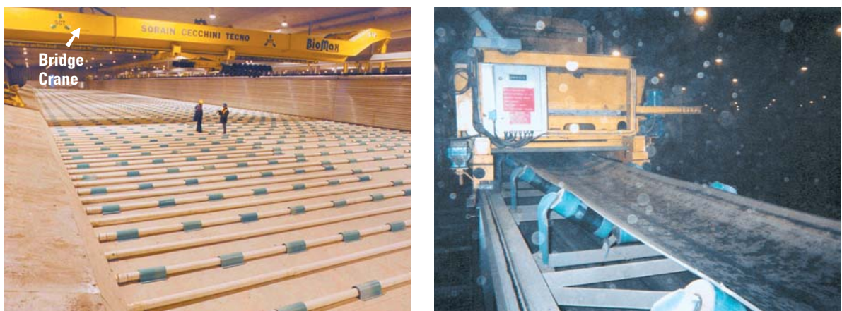
Photo 3-15: Edmonton aeration hall (before facility operation) and closeup of the conveyor and sidecar system Edmonton employs a mechanized approach to the air-floor composting process. Conveyors and sidecars (above right) automatically load the bays with immature compost. Three separate bridge cranes (like the one shown above left) straddle each bay and move up and down its length.
