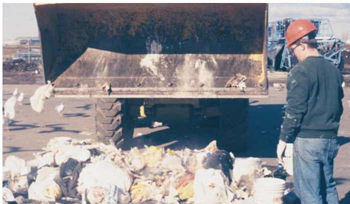
Photo 1-2: Removing samples for waste characterization Under supervision of the sampling coordinator, a front-end loader removed one to two samples from each pile.
