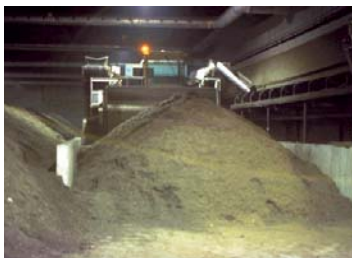
Photo 3-9: Automated windrow turner at the Conporec facility
