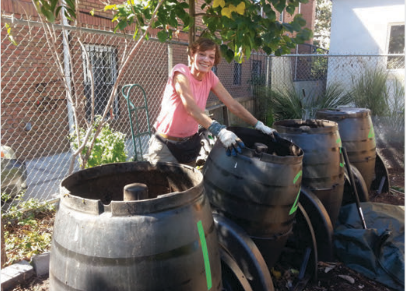
Compost for Brooklyn currently processes organic waste using a four-bin tumbler composting system. It's considering alternative composting systems to expand its capacity.
