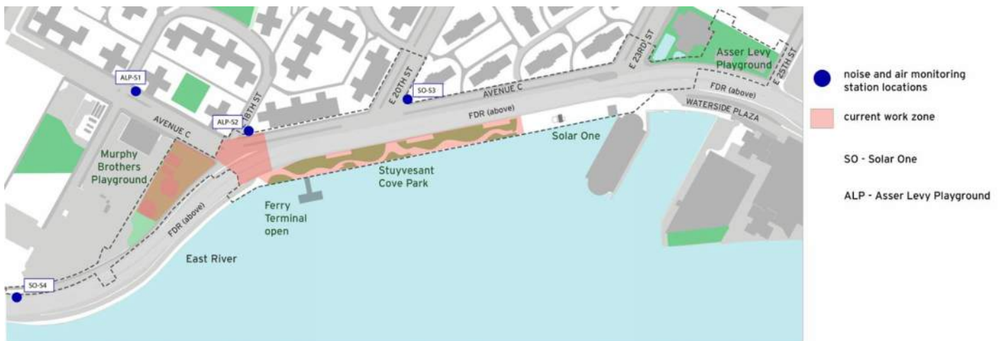
Fig.3B ESCR Project Area 2 Phase 3 Air Quality Monitoring Station Locations, as of March 22 nd , 2023
