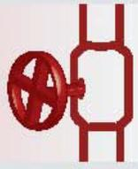
Combination standpipe valve handles must be painted **yellow**.
