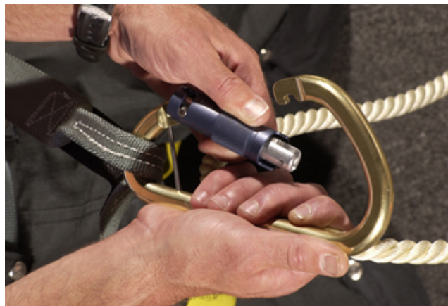
Push Gate Towards Solid Part of Hook
