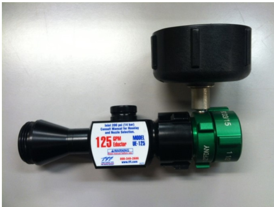
Figure 5: Educator incorrectly assembled
