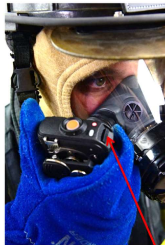
SCBA Mask – Place RSM DIRECTLY on Voicemitter
