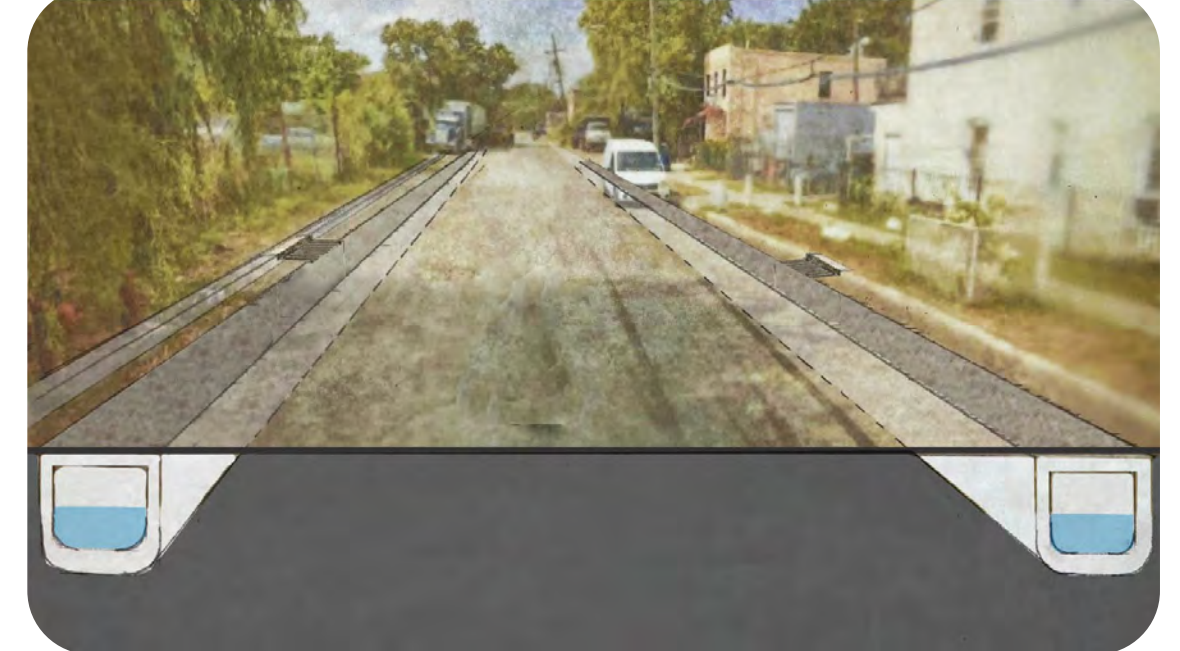
The new storm sewers will rely on innovative sewer system design using channels in the street surface (above) or box sewers under the street (below).
