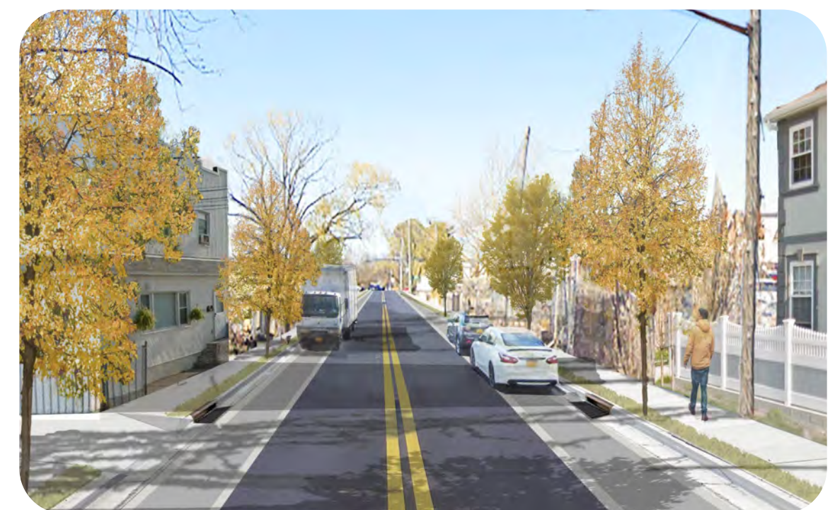
Illustration of Ruby Street with new roadway, sidewalks and at-grade drainage channels under the parking lane.
