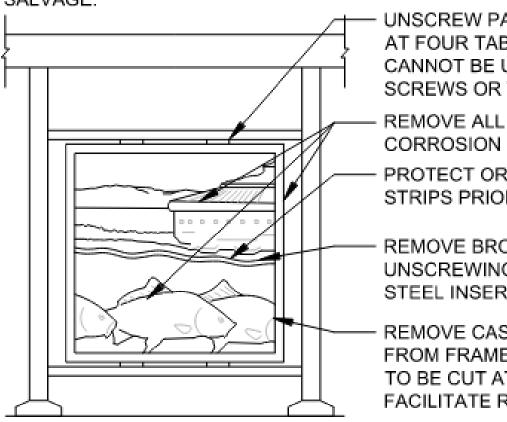
UNSCREW PANELS FROM FENCE AT FOUR TABS, IF SCREWS CANNOT BE UNSCREWED. SCREWS OR TABS MAY BE CUT
