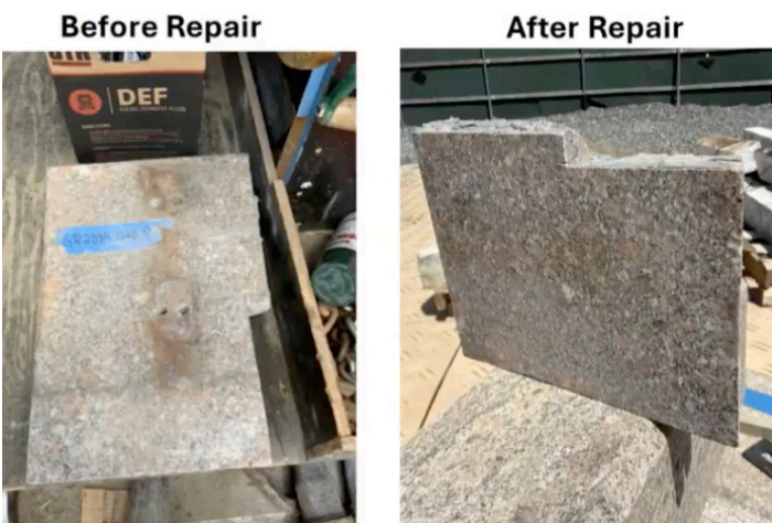
Image: The project team salvaged and cleaned granite elements for project reuse.
