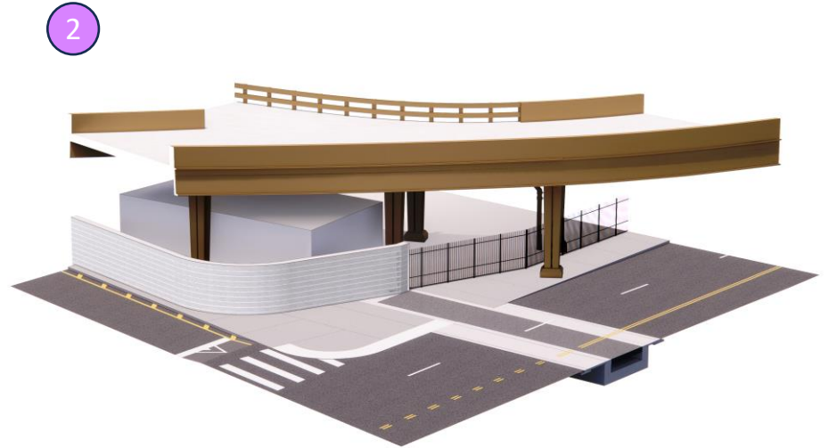
Rendering of floodwall tie-in and flip-up gate at South Street under Brooklyn Bridge From 2021 PDC Presentation :
