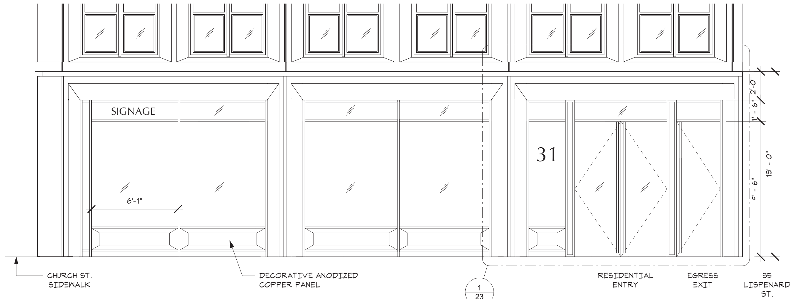
1 ENLARGED ELEVATION_ LISPENARD ST. 1/4" = 1'-0"
