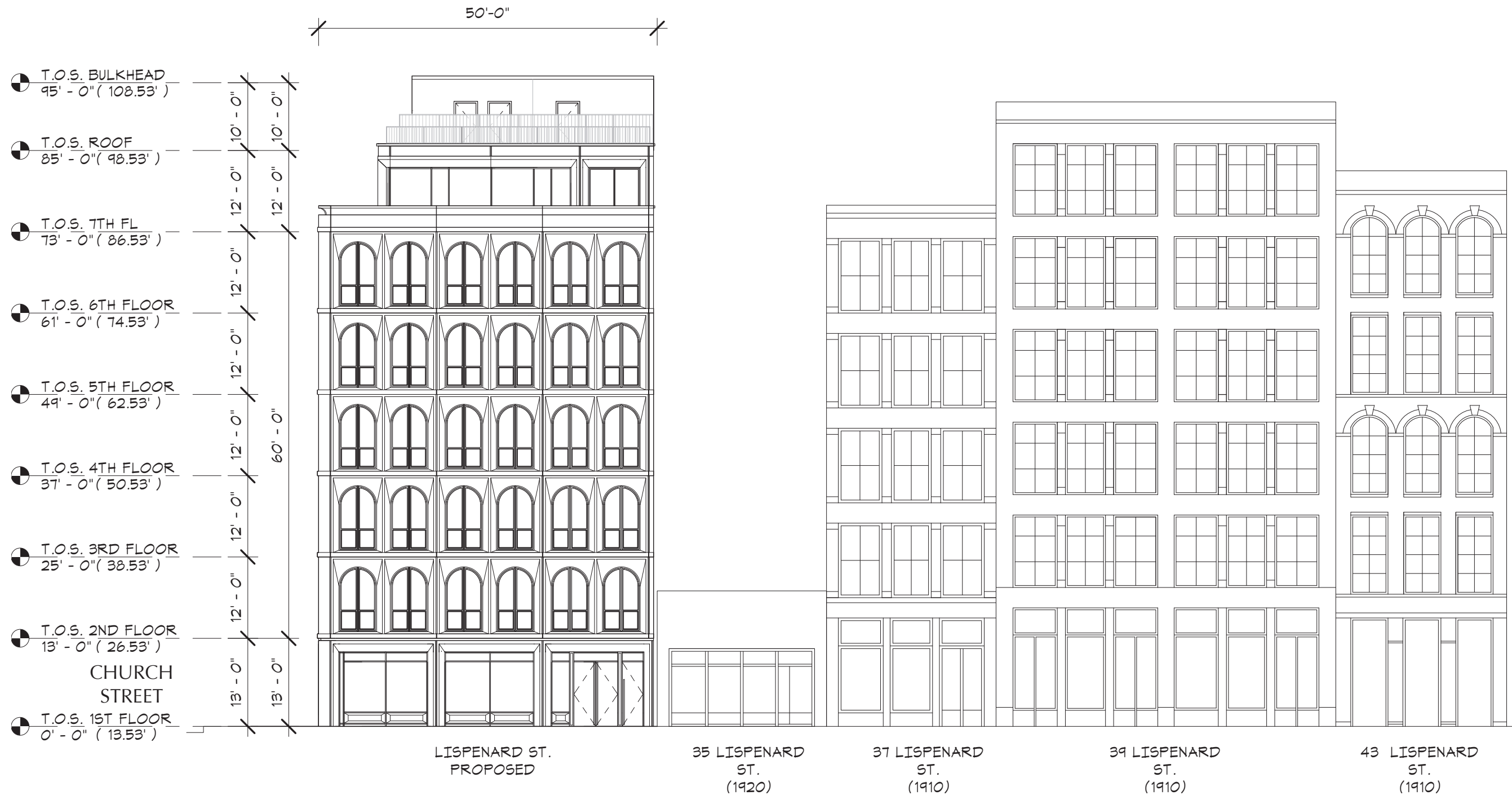
① SOUTH ELEVATION 1/16" = 1'-0"
