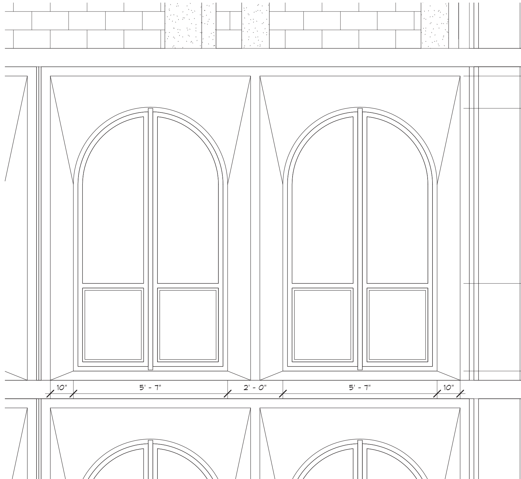
② ENLARGED ELEVATION_ CHURCH ST. 1/2" = 1'-0"
