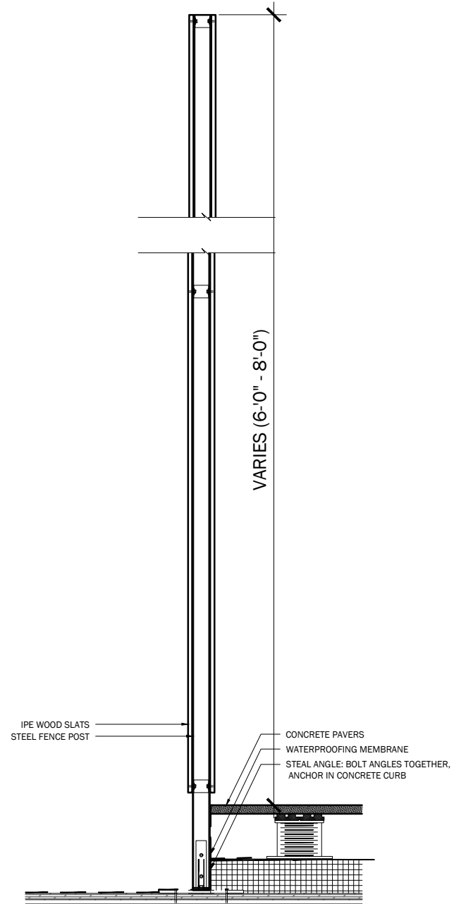
1 | PROP. WOOD FENCE AS MECH. SCREEN SECTION | 3/4" = 1'-0"
