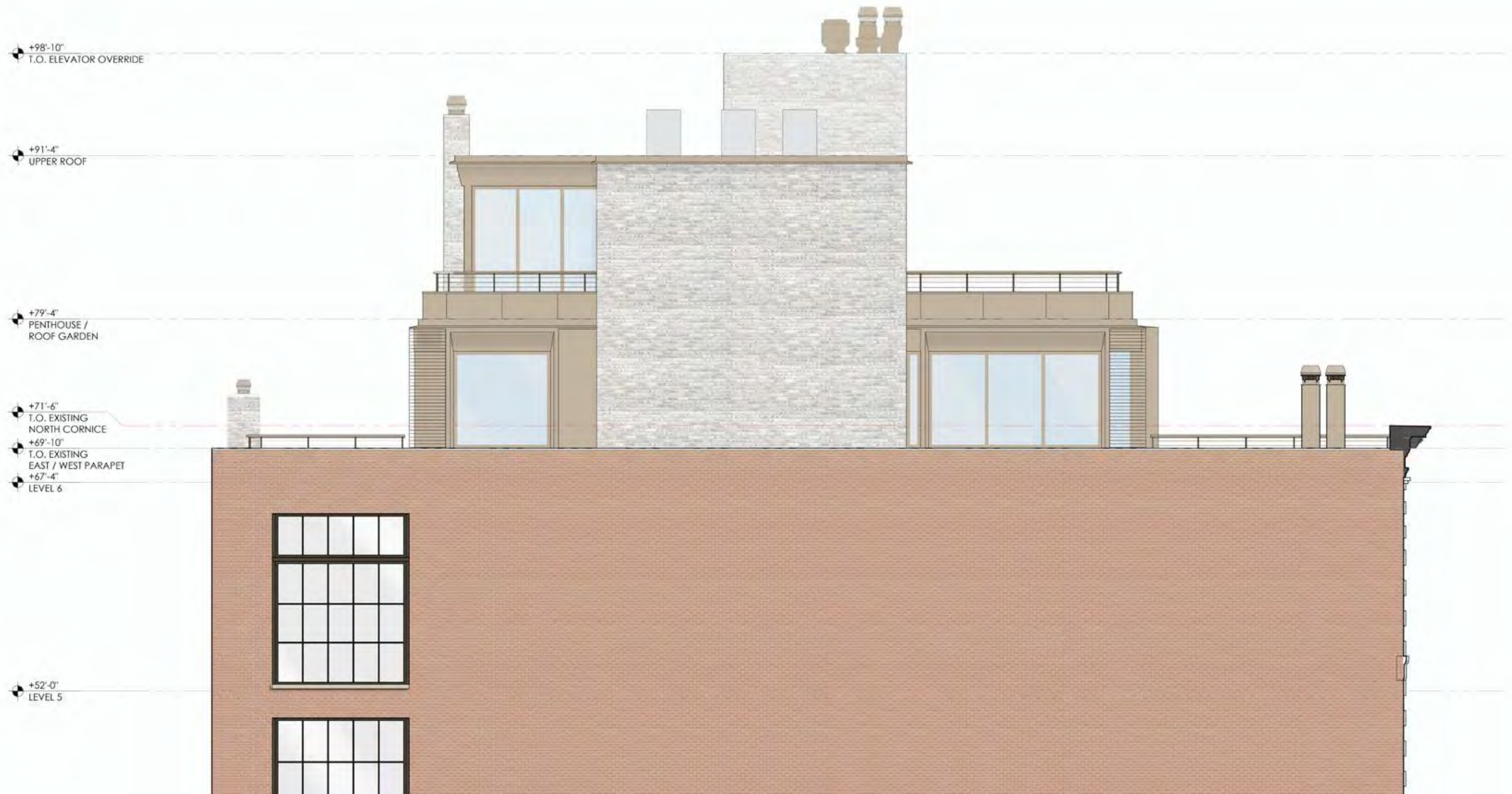
Proposed 6th Floor & Penthouse enlarged east elevation
