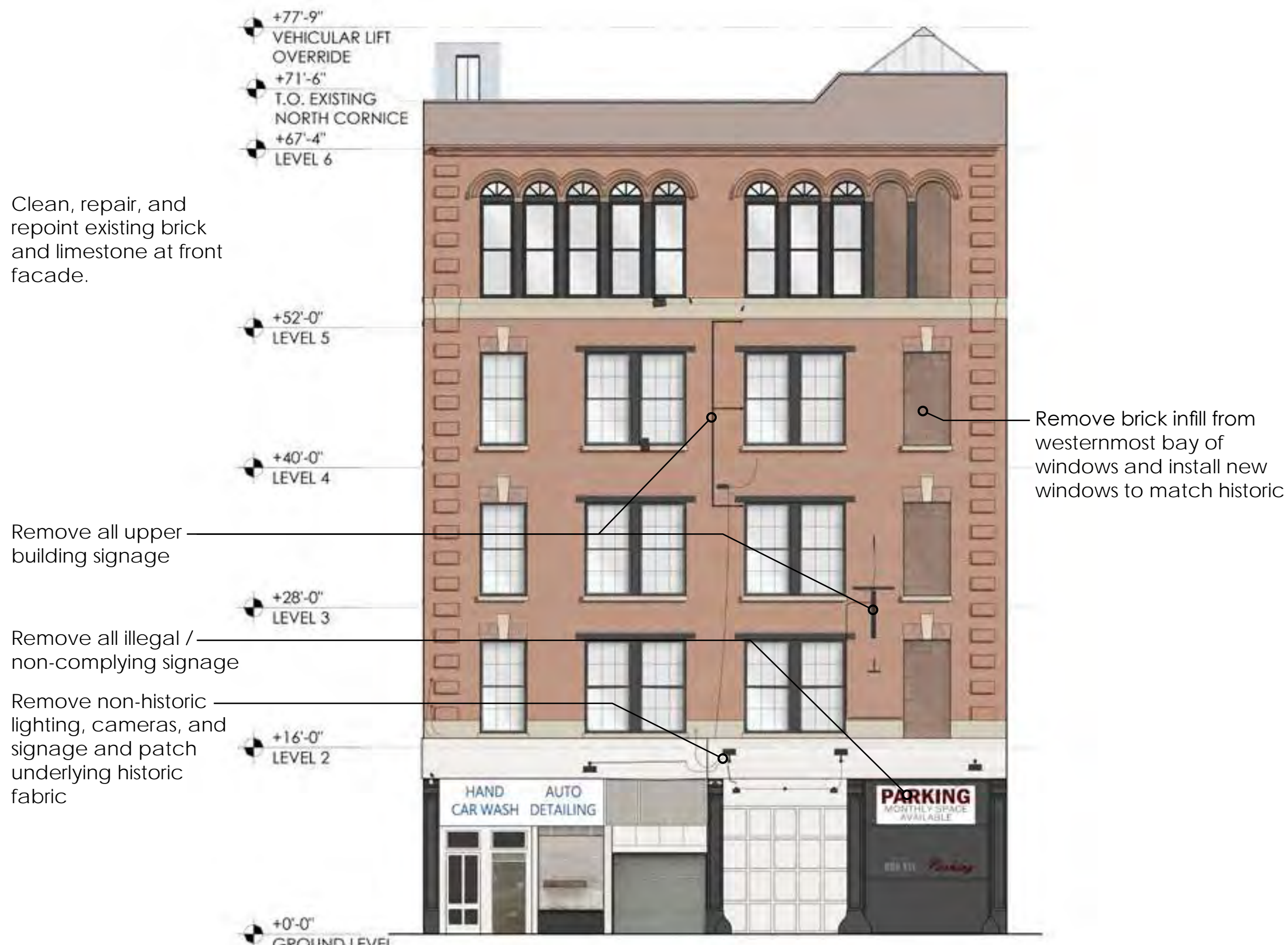
Existing North Elevation
