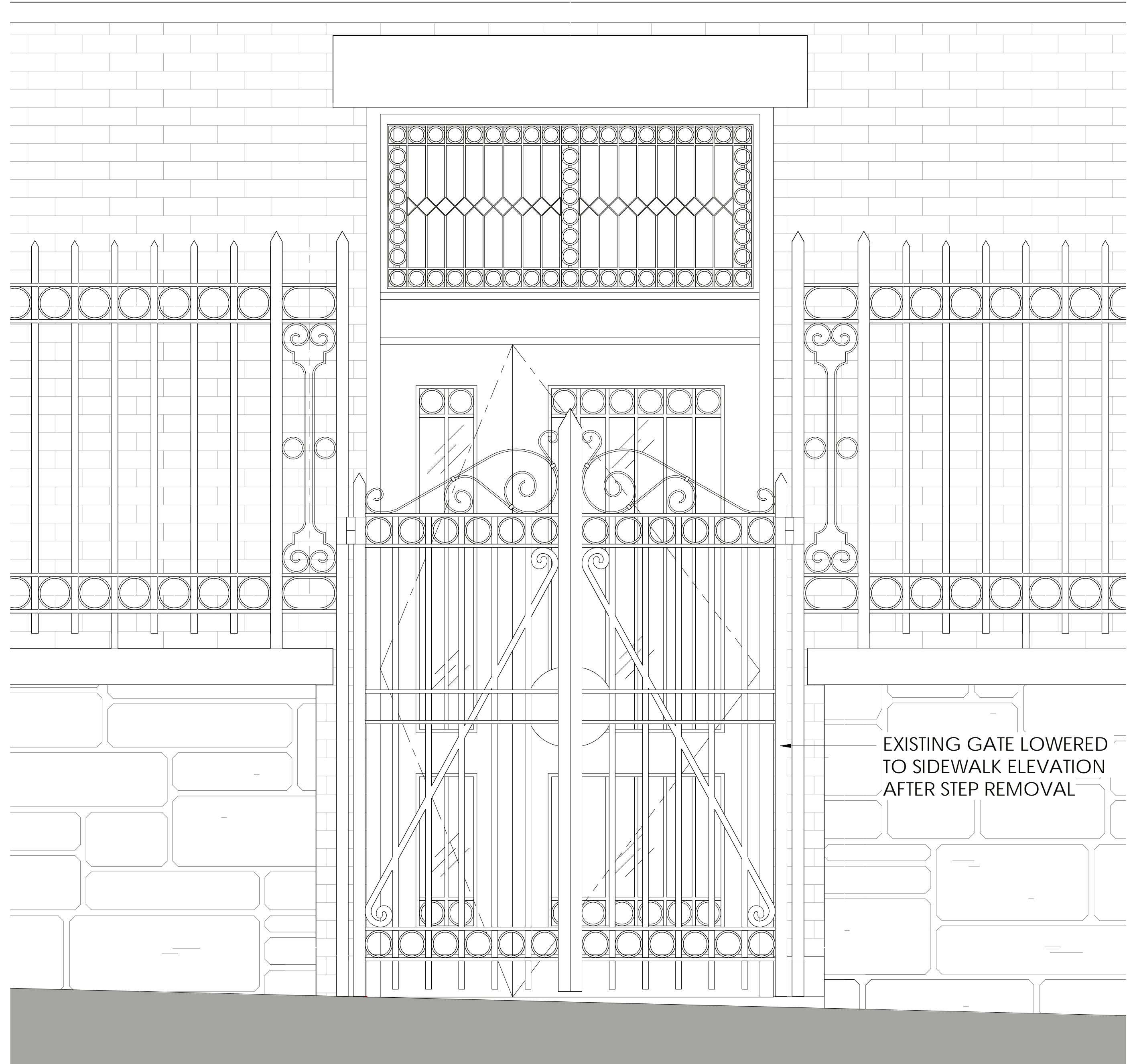
RESTORATION WORK - ON EXISTING 64TH ST ENTRANCE GATE
