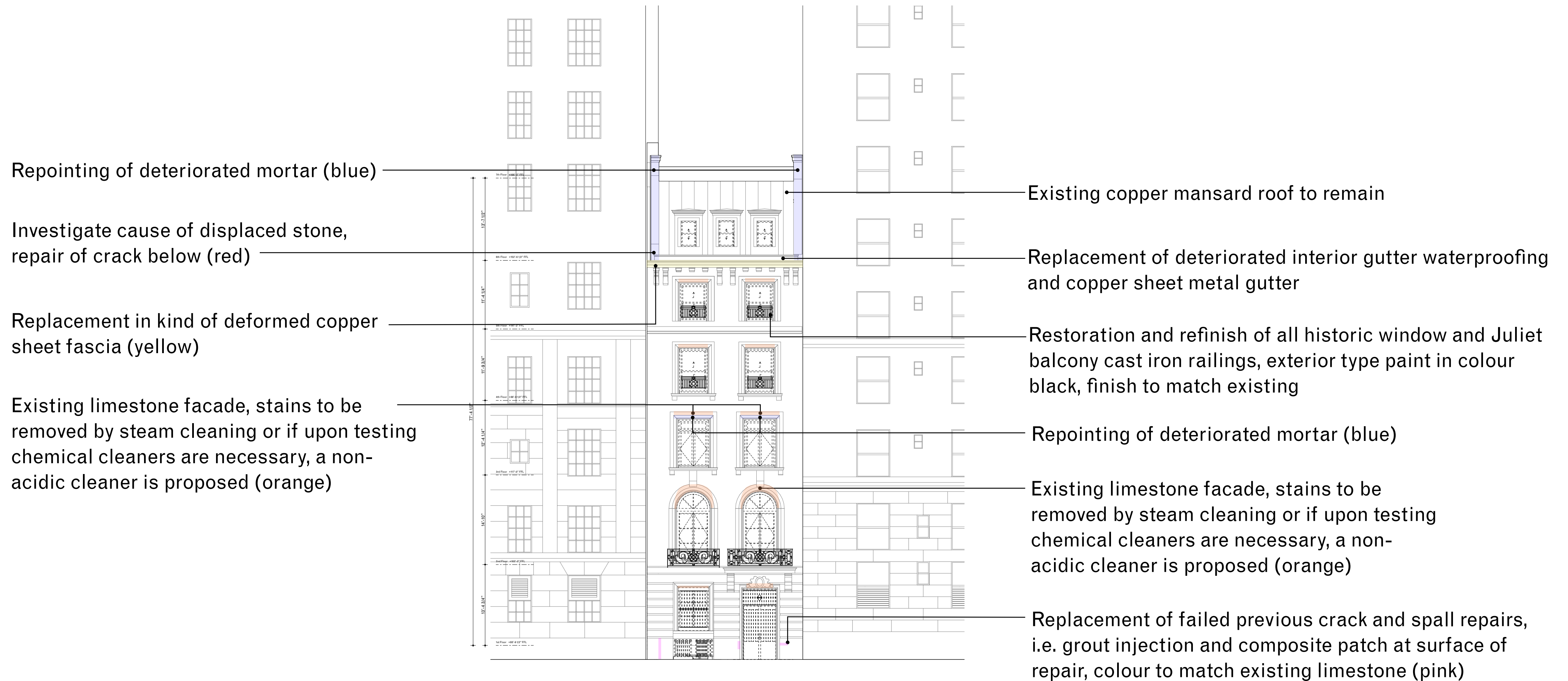
Existing West elevation
