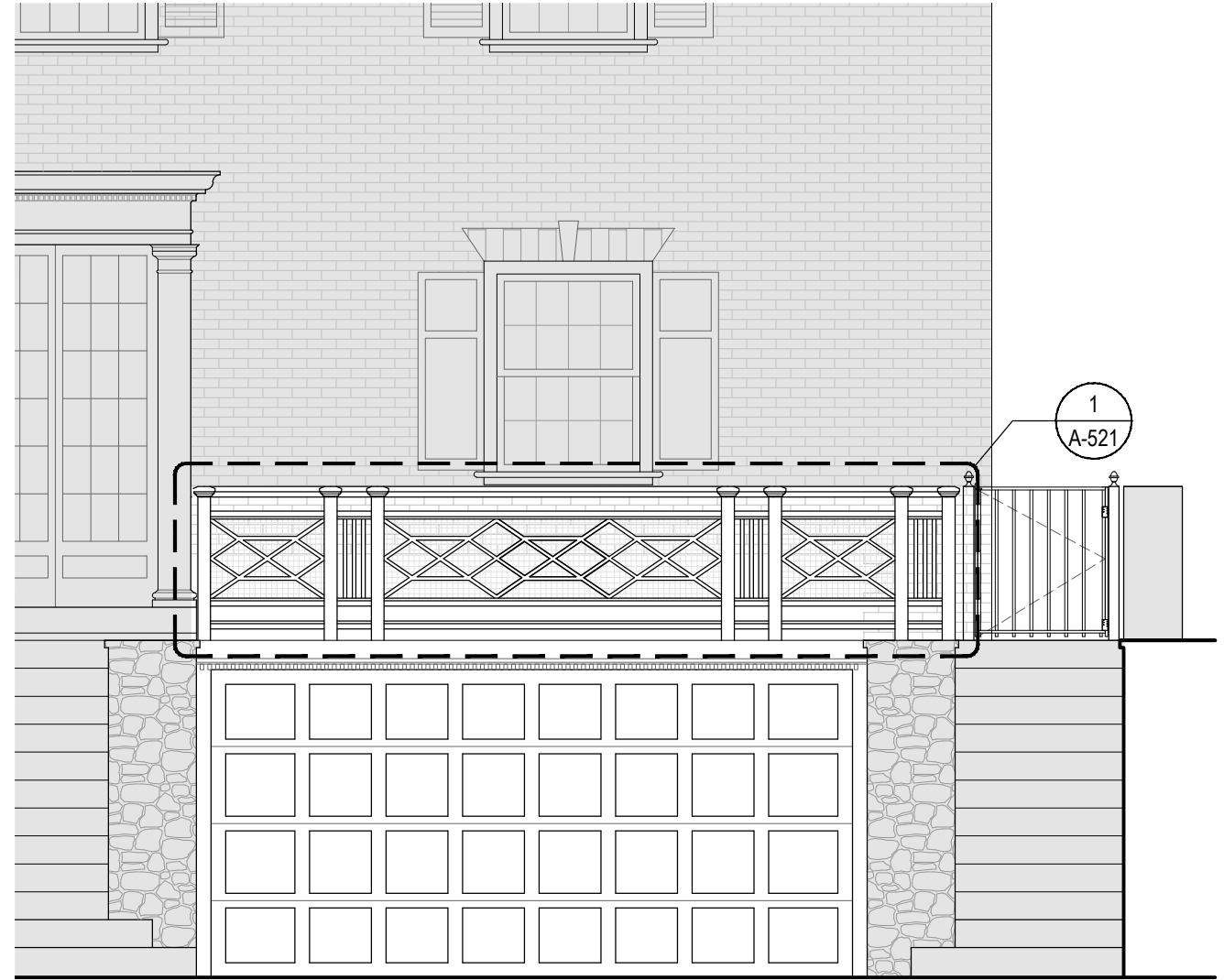
PROPOSED WALKABLE ROOF AND RAILING
