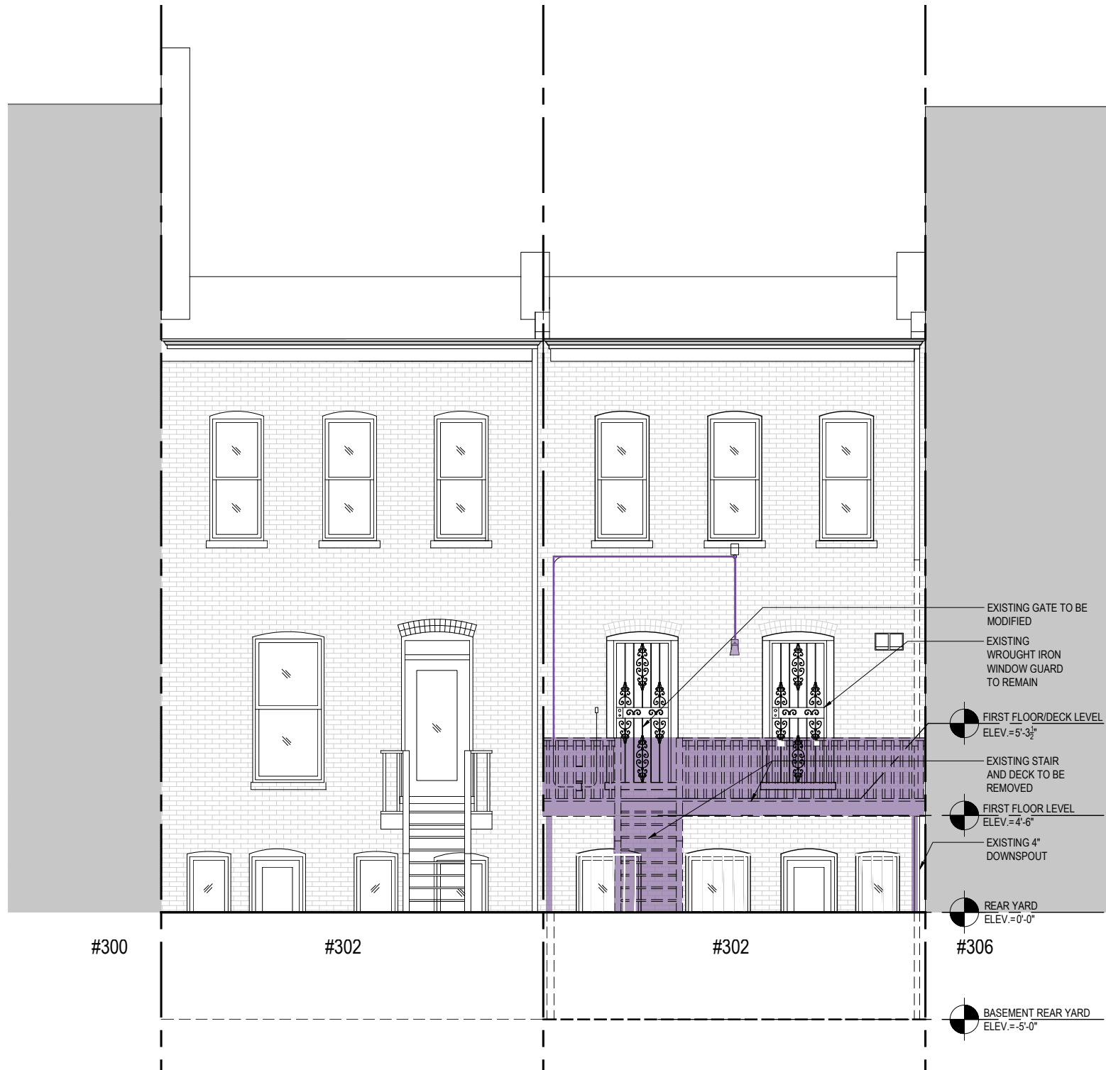
1 | REAR ELEVATION - EXISTING/REMOVALS
