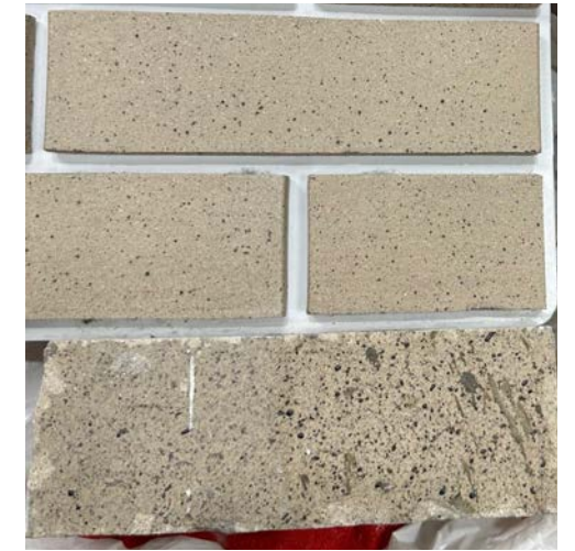
EXISTING BRICK COLLECTED FROM PROBES
