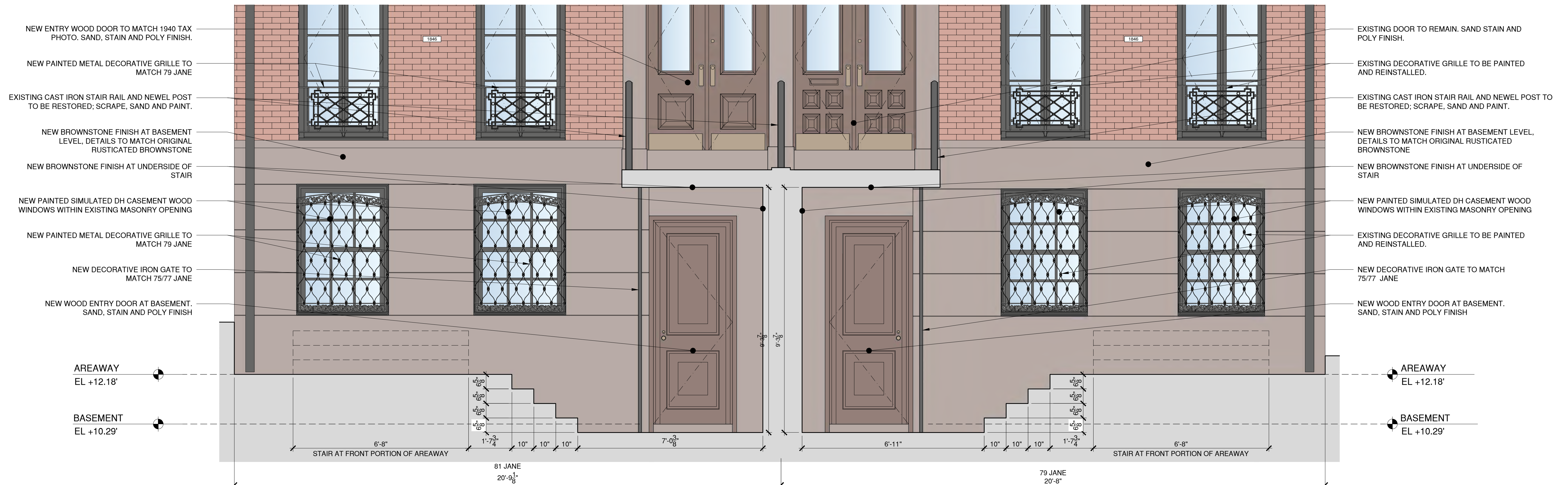
2 PROPOSED AREAWAY & STOOP SECTION SCALE: 1/2" = 1'-0"
