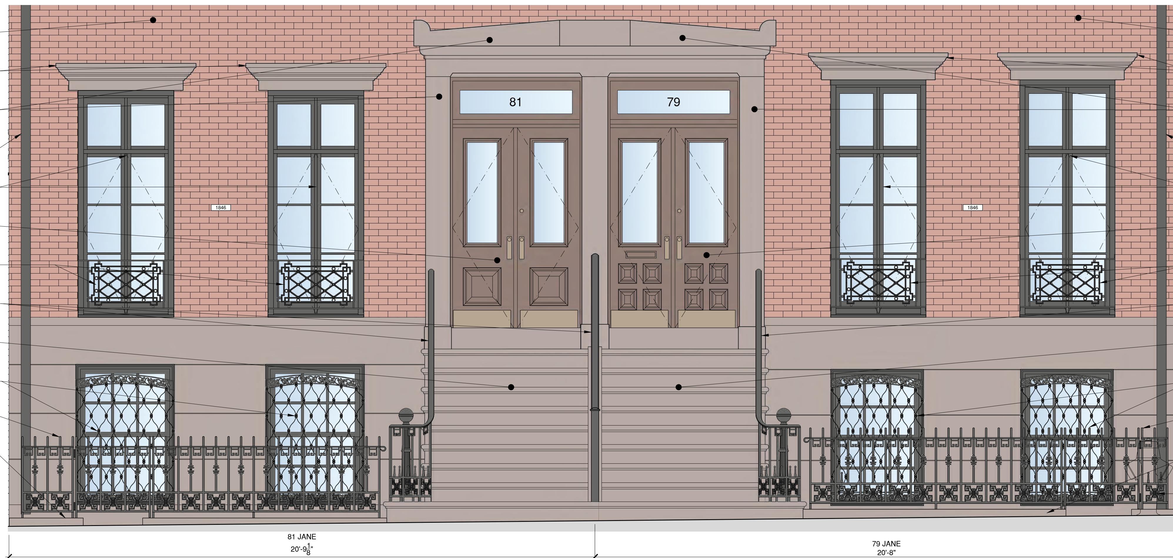
2 PROPOSED AREAWAY & STOOP SECTION SCALE: 1/2" = 1'-0"
