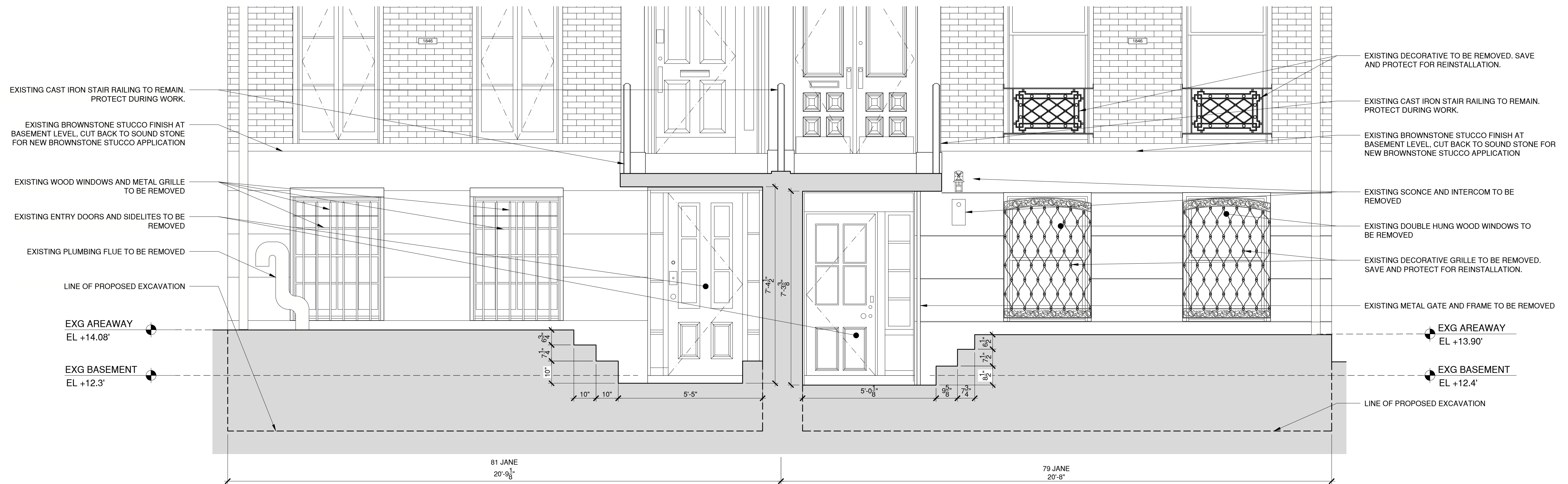
1 EXISTING / DEMOLITION AREAWAY & STOOP SECTION SCALE: 1/2" = 1'-0"
