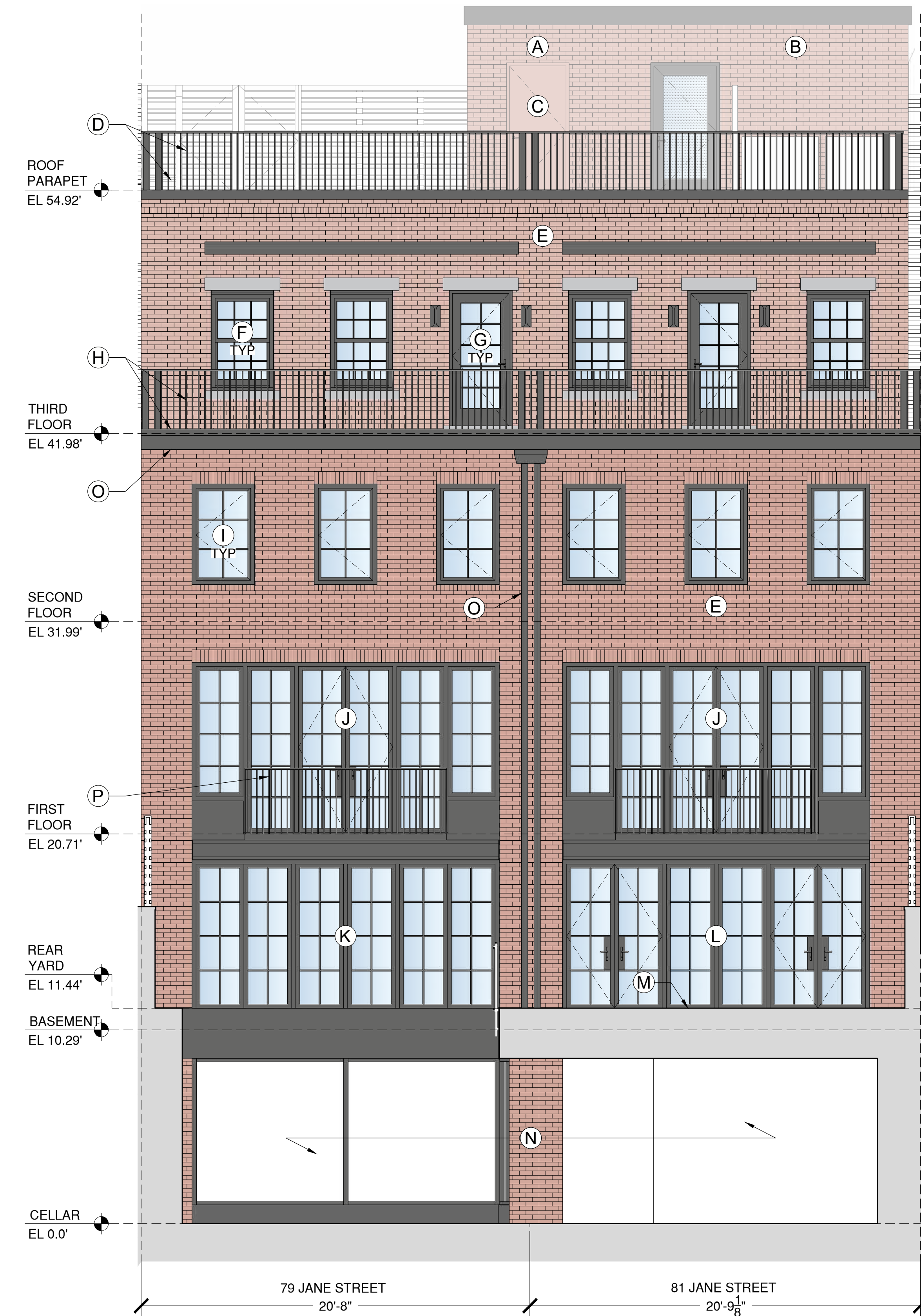
② PROPOSED REAR ELEVATIONS SCALE: 1/4" = 1'-0"
