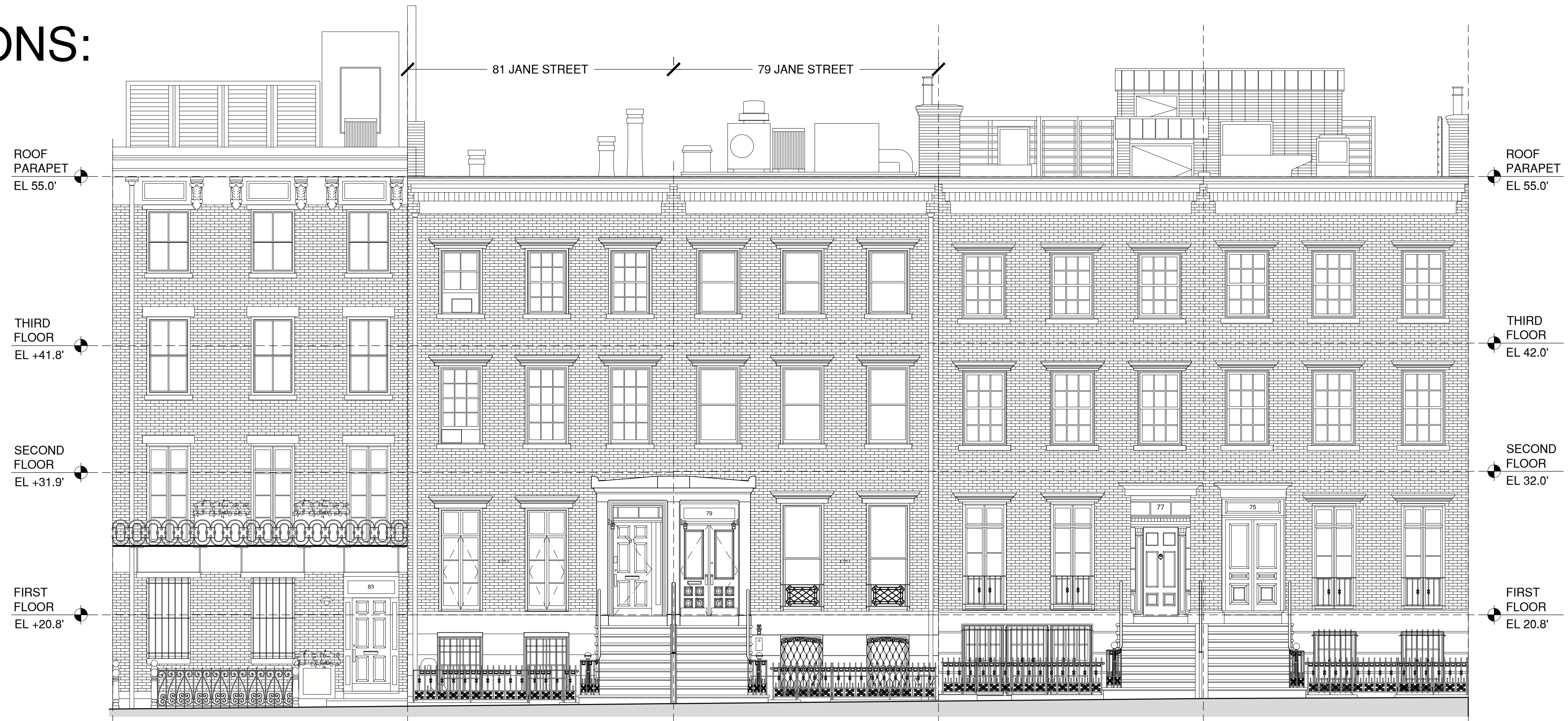
① EXISTING / DEMOLITION FRONT ELEVATION SCALE: 3/16" = 1'-0"
