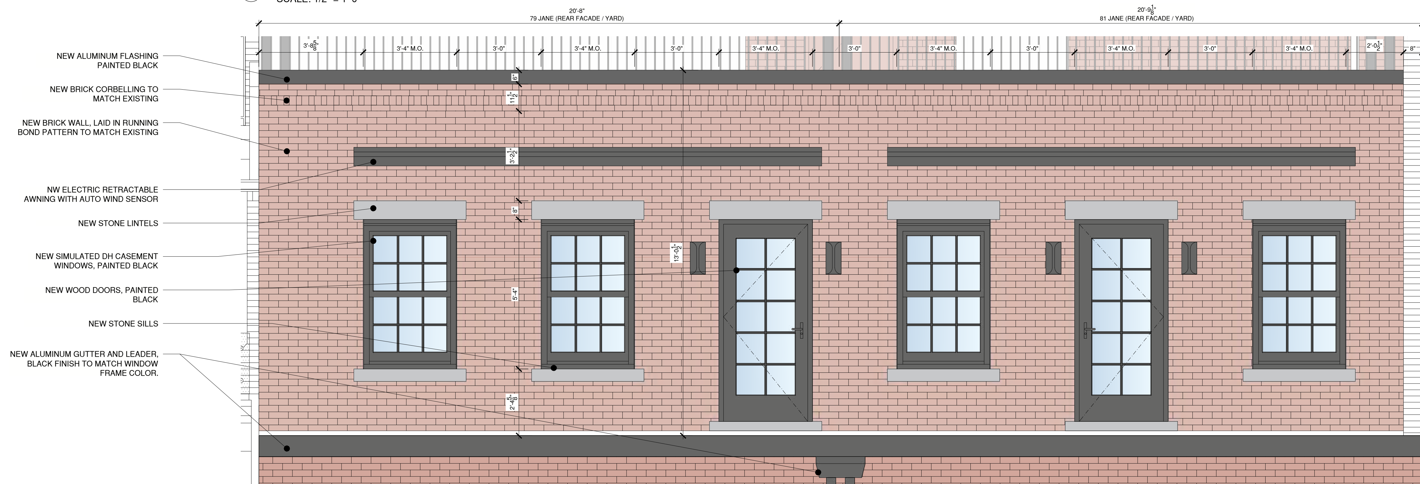
2 PROPOSED REAR FACADE ELEVATION 79/81 JANE - THIRD FLOOR SCALE: 1/2" = 1'-0"
