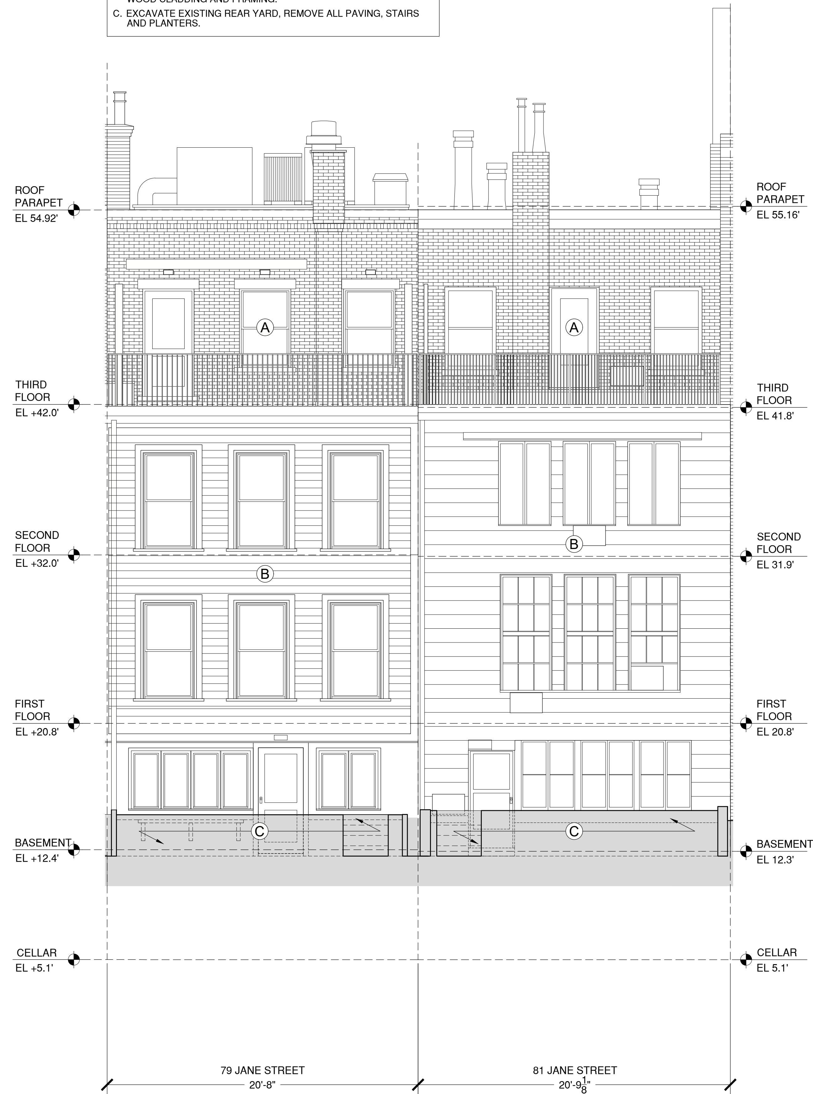
① EXISTING / DEMOLITION REAR ELEVATIONS SCALE: 1/4" = 1'-0"
